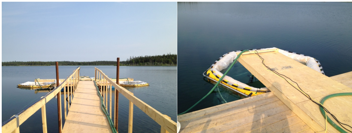
Figure 3 Limnocorrals Used for the Nero Lake Water Treatment Pilot Trial
