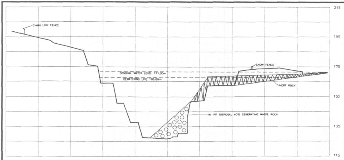
After all of the waste rock had been placed into the open pit, the upper 0.5 metres of the ramp was excavated and placed into the open pit. This was done to ensure that all the waste rock that spilled onto the ramp was placed in the open pit. It appeared that the majority of the waste rock had been successfully placed into the deepest cut of the open pit. This was determined by measuring the depth of the disposal area at the open pit with a depth indicator.
