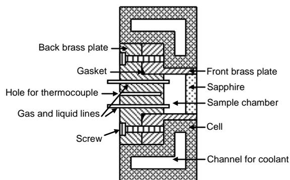
Figure 1: Schematic of the high-pressure Raman cell
