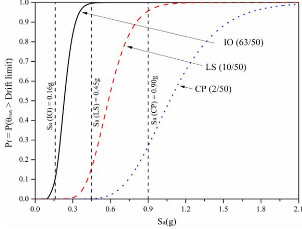
Figure 3: Peak displacement fragility curves of the hybrid shear wall with  $K_r = 2.5$
