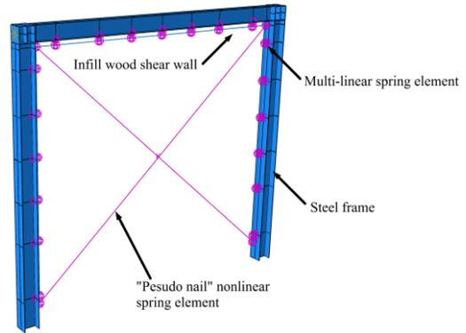
Figure 2: FE model for timber-steel hybrid shear wall system.
