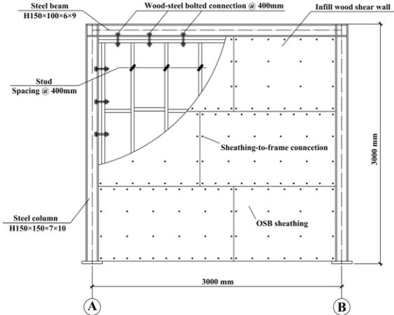
Figure 1: Configuration of baseline timber-steel hybrid shear wall.
