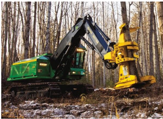
Figure 1. 953K Tracked Feller Buncher from John Deere shown in operation (John Deere, 2018).
