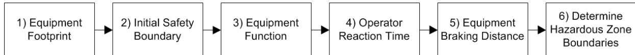
Figure 2: Steps for determining the hazardous zone around a piece of construction equipment
