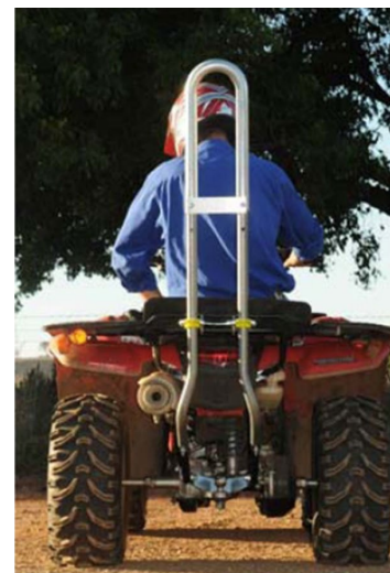
Figure 5: Example of Rollover/Crush Protection Device attached to the rear of an ATV
