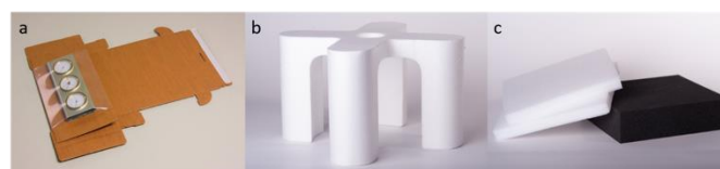
Figure 1. Conventional cushioning solutions a) retention pack, b) EPS c) EPU and EPE.
