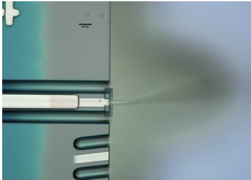
Figure 2.15: Micrograph of PWB connect SOA to SiP chip - focus on SOA on non-angle side
