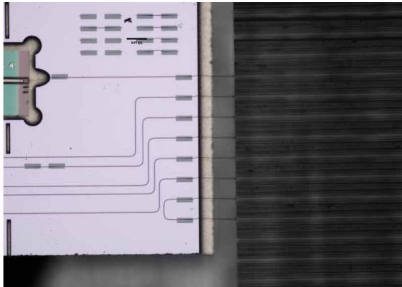
Figure 2.11: Micrograph of fabricated device – fiber array assembly on right side
