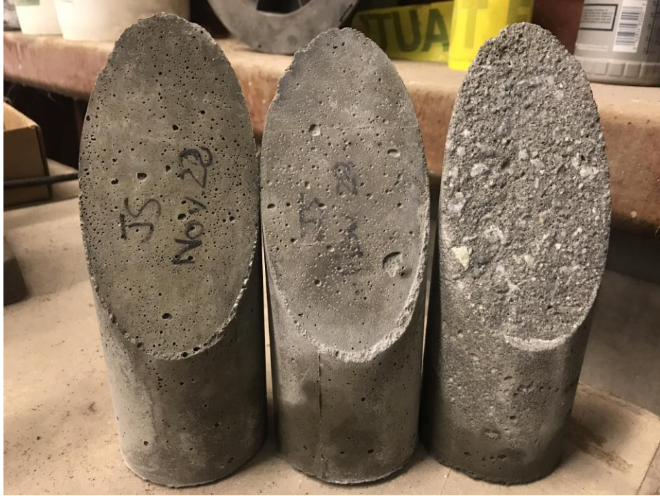
Figure 4: [From left-to-right] As-Cast Specimen, Wirebrushed Specimen, and Sandblasted Specimen
