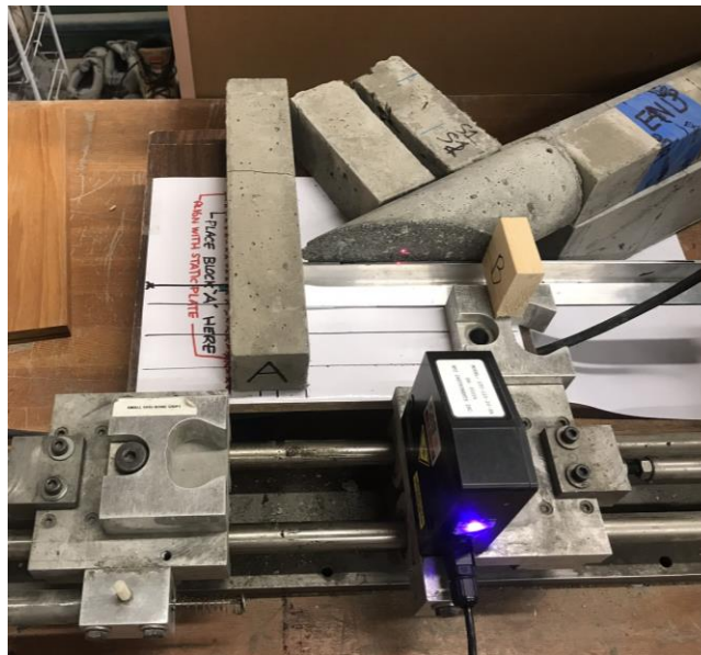
Figure 6: Laser Profilometry Set-Up for Roughness Quantification
