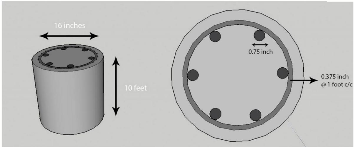
Figure 2-4: RC column example
