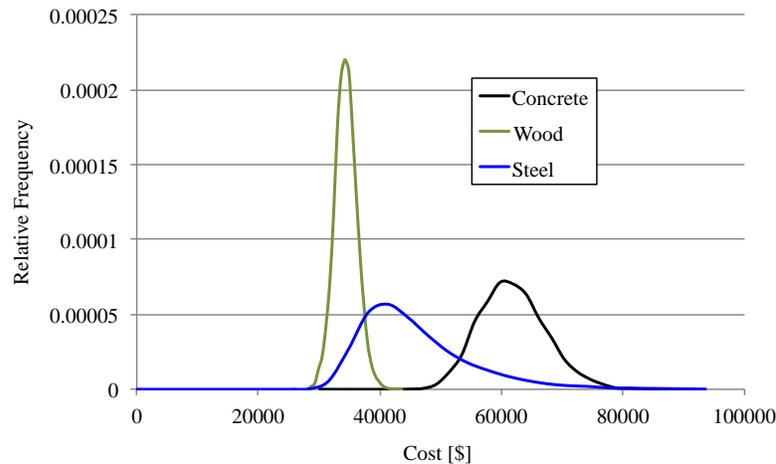
Figure 5-3: Relative frequency diagrams for total lifecycle cost
