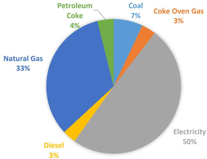
Figure A-4: Average energy usage in extraction & manufacturing phase
