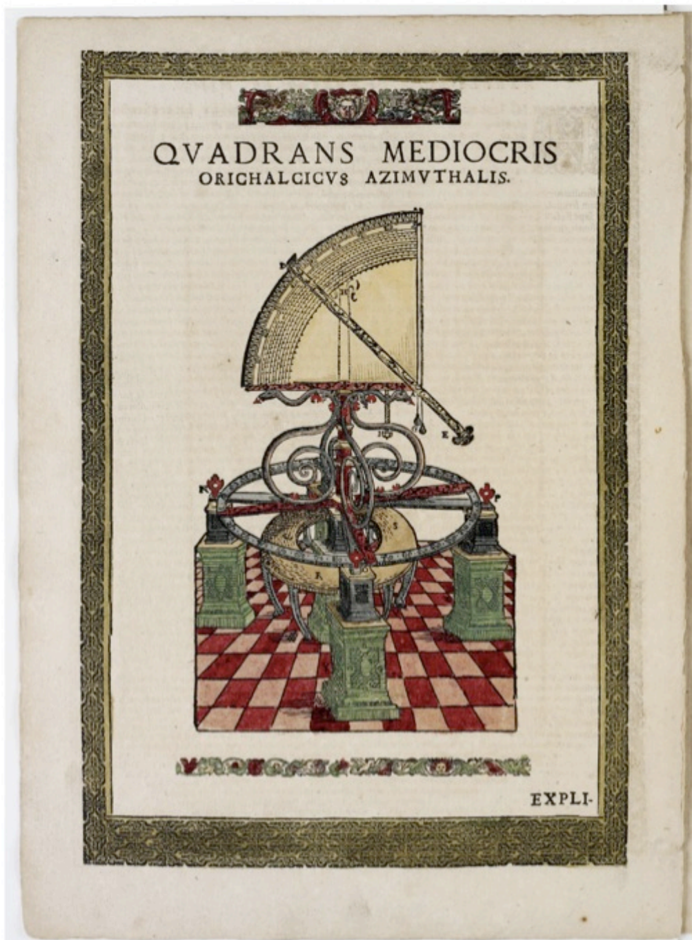
Figure 44 Medium Sized Azimuth Quadrant of Brass , from Tycho Brahe, Astronomiae instauratae mechanica , 1598, woodblock print on paper and gouache. The National Library of Denmark and the University Library of the University of Copenhagen. Picture with permission from The Royal Library Copenhagen.
