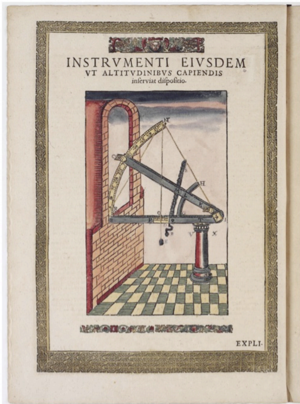
Figure 45 Sextant Mounted for the Observation of Altitudes , from Tycho Brahe, Astronomiae instauratae mechanica , 1598, woodblock print on paper and gauche. The National Library of Denmark and the University Library of the University of Copenhagen. Picture with permission from The Royal Library Copenhagen.
