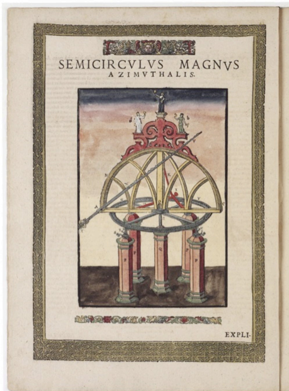
Figure 48 Great Azimuth Semicircle , from Tycho Brahe, Astronomiae instauratae mechanica , 1598, woodblock print on paper and gouache. The National Library of Denmark and the University Library of the University of Copenhagen. Picture with permission from The Royal Library Copenhagen.
