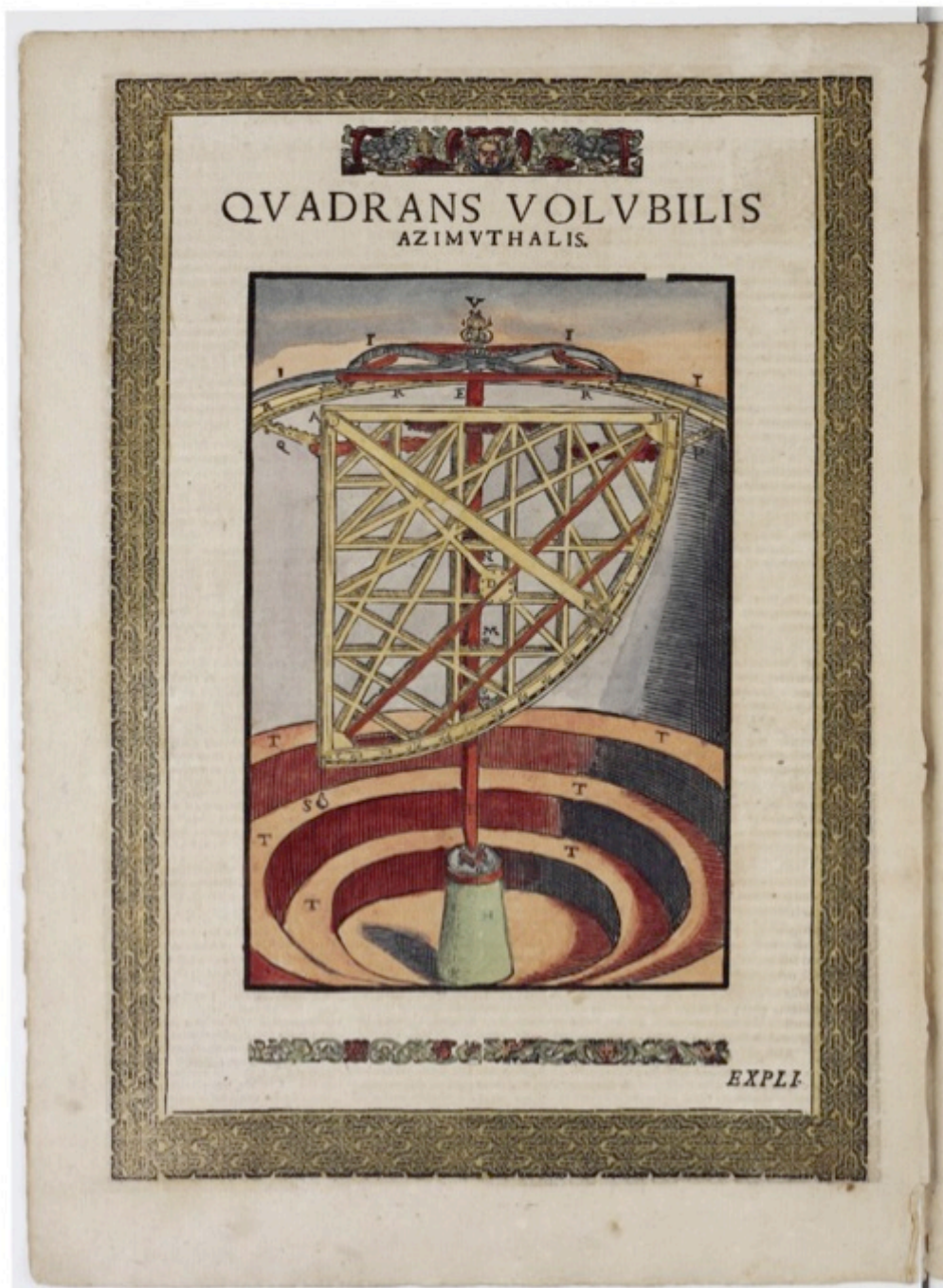
Figure 46 Revolving Azimuth Quadrant , from Tycho Brahe, Astronomiae instauratae mechanica , 1598, woodblock print on paper and gouache. The National Library of Denmark and the University Library of the University of Copenhagen. Picture with permission from The Royal Library Copenhagen.
