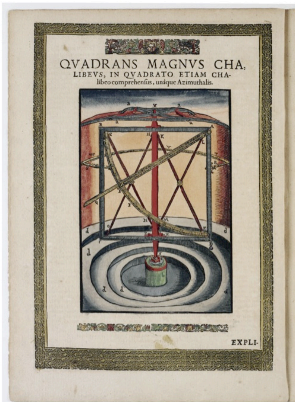
Figure 47 Great Steel Quadrant , from Tycho Brahe, Astronomiae instauratae mechanica , 1598, copper-plate engraving on paper and gouache. The National Library of Denmark and the University Library of the University of Copenhagen. Picture with permission from The Royal Library Copenhagen.
