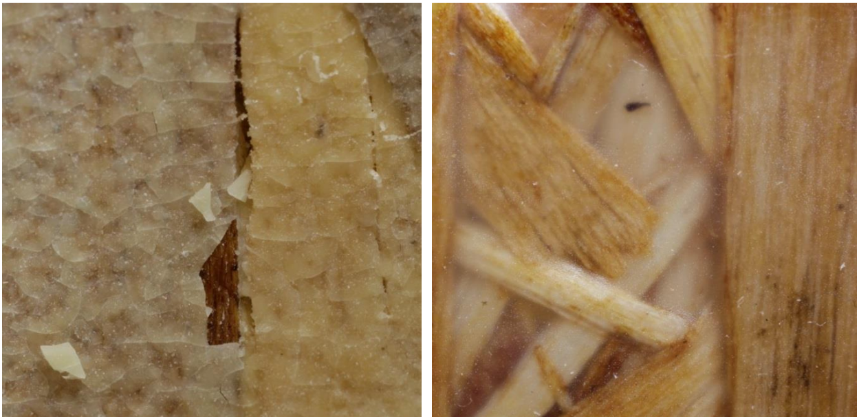
Figure 4.6. Close up of the surface of OSB sprayed with approximately 270 \text{ g / m}^2 of molten carnauba (left) wax and Vaseline (right). Note that the high application rate caused surface coatings to form, even though the OSB samples were hot ( 170^\circ\text{C} ) when the waxes were sprayed onto them. Carnauba wax coatings cracked and flaked off when touched, while Vaseline formed a defect-free coating that filled the surface voids
