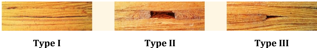
Figure 2.5. Three types of inter-strand voids in flakeboard, as classified by Furuno et al. (1983)
