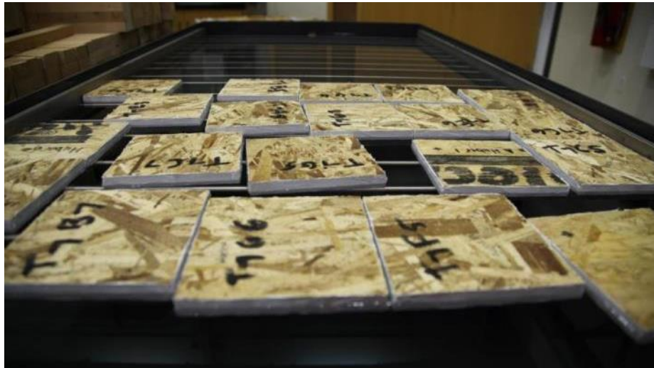
Figure 5.1. Samples were floated face down on water for 72 h. The weight and the thickness of each sample was measured after 2 h, 24 h, 48 h, and 72 h
