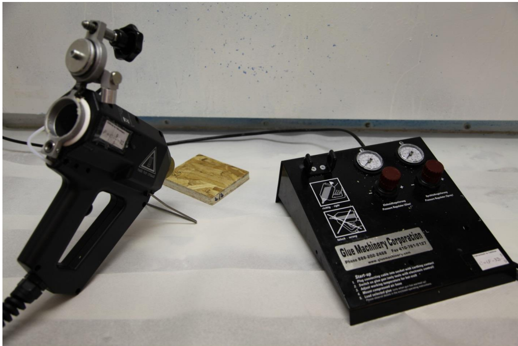
Figure 4.3. The Champ 10s pneumatic spray gun used to spray molten wax onto the OSB samples. Solid wax is inserted into the temperature controlled heating chamber at the back of the spray gun (left). The control panel (right) is used to set the pressure inside the heating chamber and spray pressure at the nozzle tip
