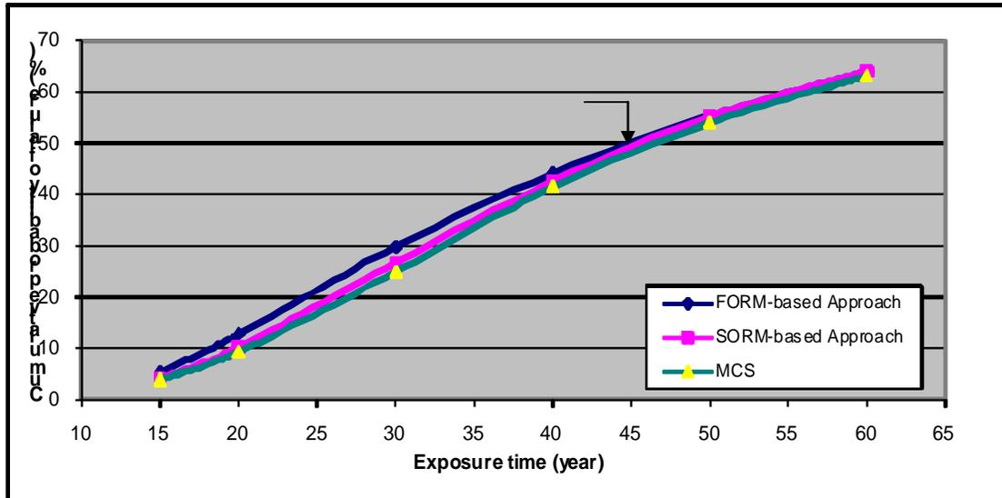
Figure 3.3. Probability of failure due to the thinness of the pipe wall caused by external and internal corrosion throughout the exposure time using MCS, and FORM- and SORM-based approaches (failure criteria of  $\sigma_{\theta} \geq \sigma_Y$ )
