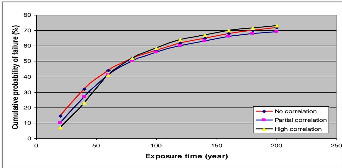
Figure 2.6. Probability of failure throughout the exposure time, for a normal distribution with different correlation assumptions using a SORM-based approach (203 mm pipe diameter and failure criteria of  $d^* \geq t_p / 2$ )
