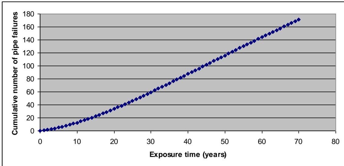
Figure 4.5. Cumulative number of pipe failures based on the results of SORM-based approach fitted to the Weibull and Exponential distributions
