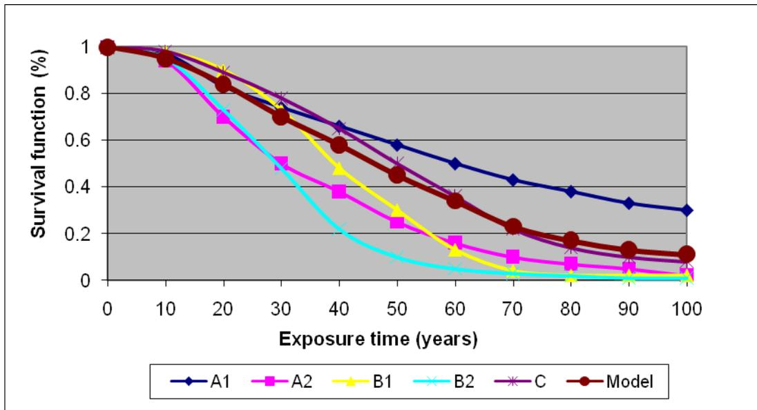
Figure 4.7. Comparing the survival functions for three municipalities with survival function associated with the Weibull Distribution using the SORM-based approach
