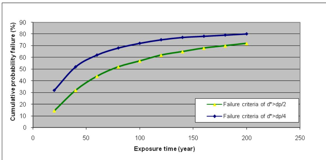
Figure 2.5. Probability of failure throughout the exposure time, for a normal distribution and two failure criteria using a SORM-based approach (203 mm pipe diameter)
