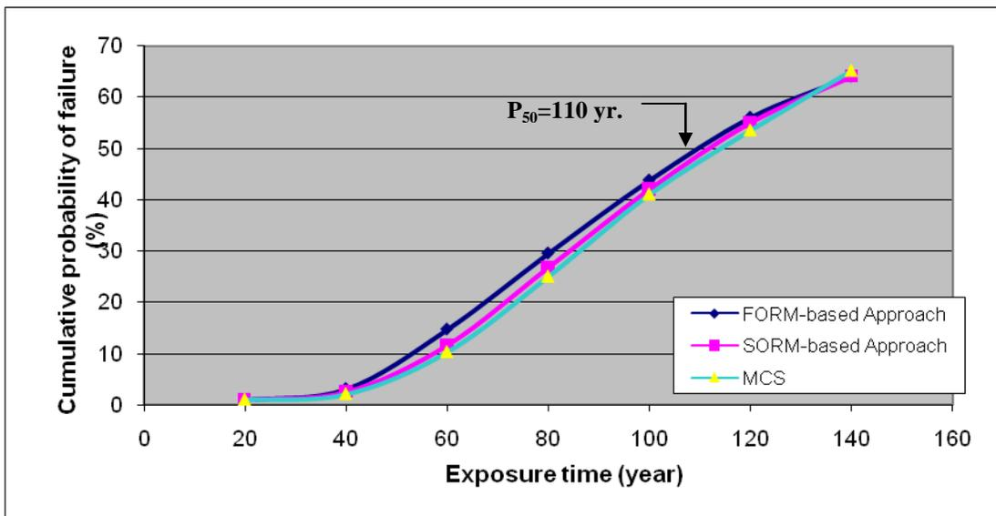
Figure3.2. Probability of failure due to the thinness of the pipe wall caused by internal corrosion throughout the exposure time using MCS, FORM- and SORM- based approaches (failure criteria of  $\sigma_F \geq \sigma_Y$ )
