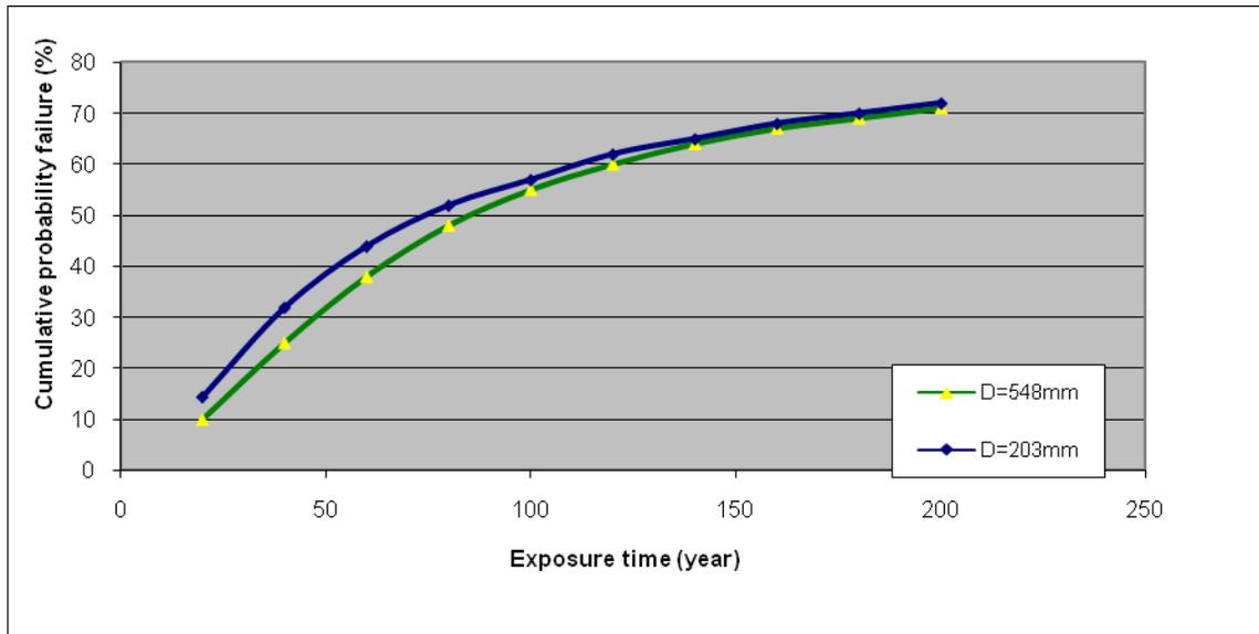
Figure 2.4. Probability of failure throughout the exposure time, for a normal distribution and various pipe diameters using a SORM-based approach (failure criteria of  $d^* \geq t_p / 2$ )
