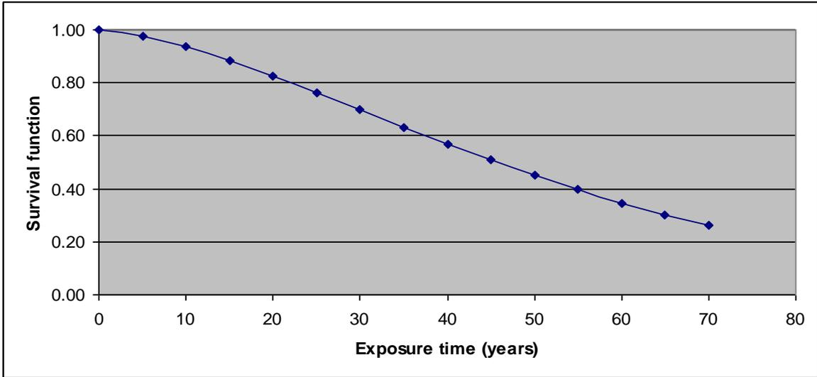
Figure 4.4 Survival function based on the hazard function for first order breaks
