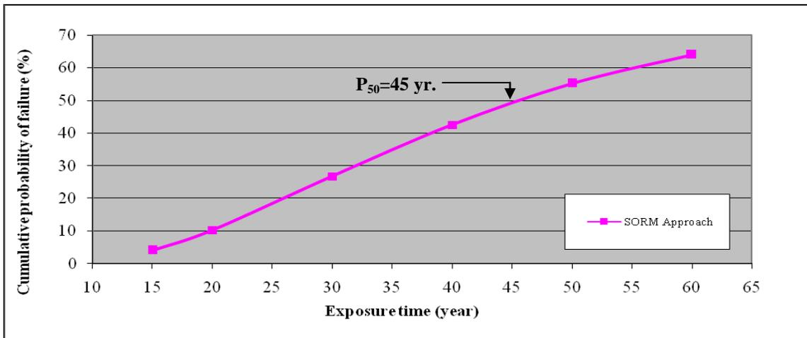
Figure 4.1. Probability of failure due to external and internal corrosion throughout the exposure time, for various statistical distributions using SORM-based approach (203 mm pipe diameter)
