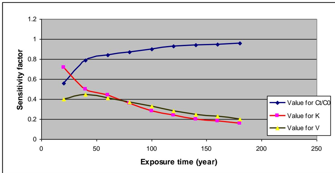
Figure 2.7. Sensitivity factors for input parameters throughout the exposure time, for a normal distribution using a SORM-based approach (203 mm pipe diameter and failure criteria of
