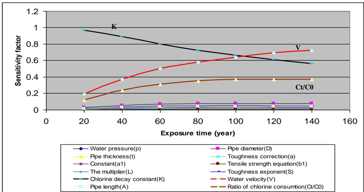
Figure 3.4. Sensitivity factors for input variables throughout the exposure time using a SORM-based approach (internal corrosion, failure criteria of  $\sigma_F \geq \sigma_Y$ )
