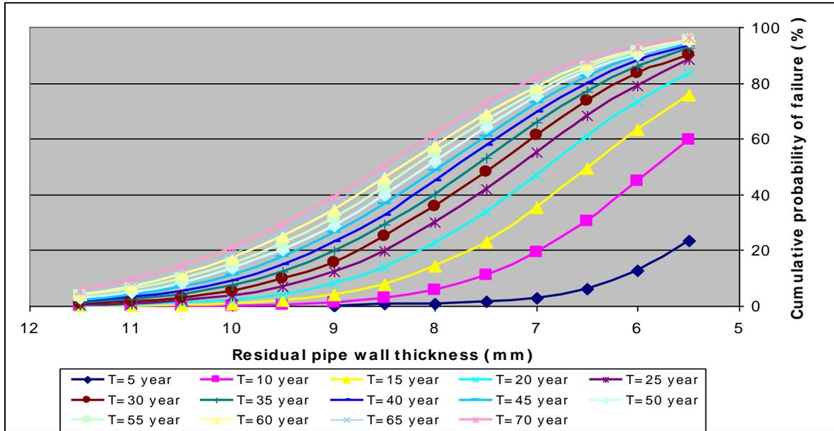
Figures 4.6. Cumulative probability of failure vs. residual pipe wall thickness, for a SORM-based approach, for different exposure times (pipe ages)
