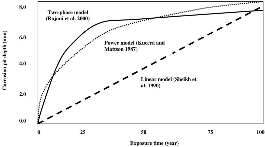
Figure 1.2. Comparison of predictive models for corrosion pit depths
