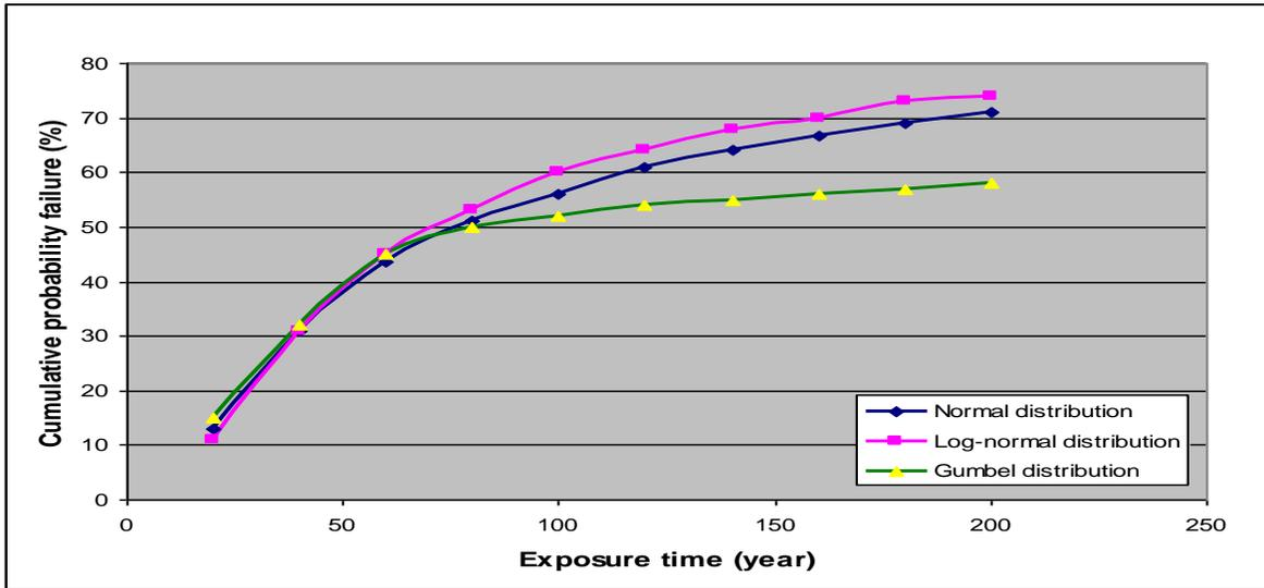
Figure 2.3. Probability of failure throughout the exposure time, for all statistical distributions using a SORM-based approach (203 mm pipe diameter and failure criteria of  $d^* \geq t_p / 2$ )
