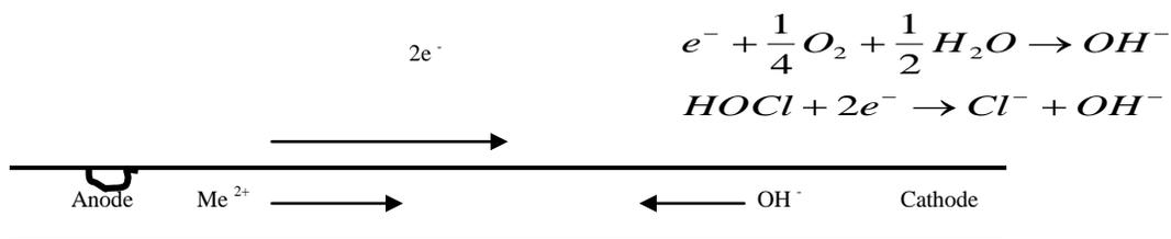
Figure 1.1. Schematic of a corrosion cell (Adapted from Snoeyink and Wagner, 1996)
