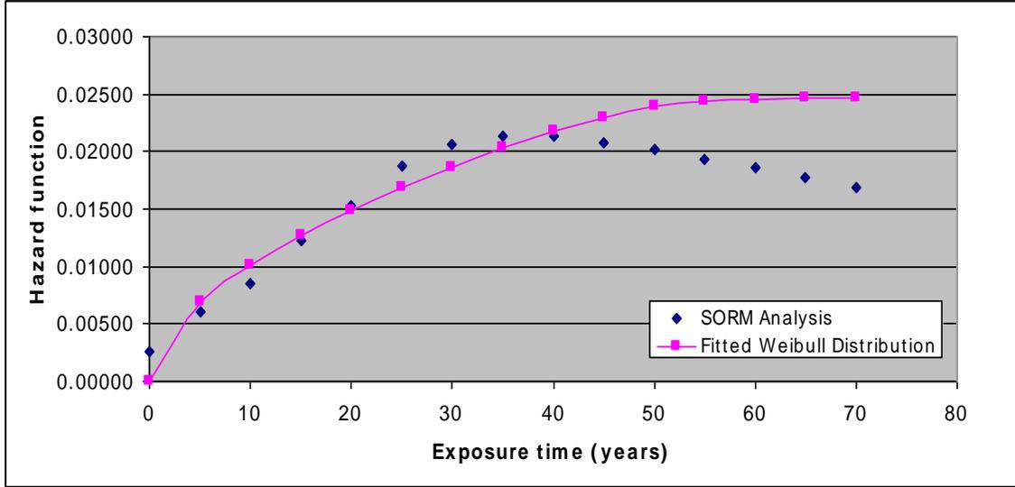
Figure 4.3. Discrete hazard function fit to the Two-parameter Weibull distribution function ( $p=1.552, k=0.017$ )
