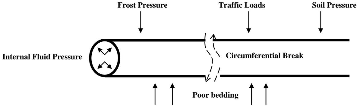
Figure1.3. Circumferential failure mode for cast iron pipe
