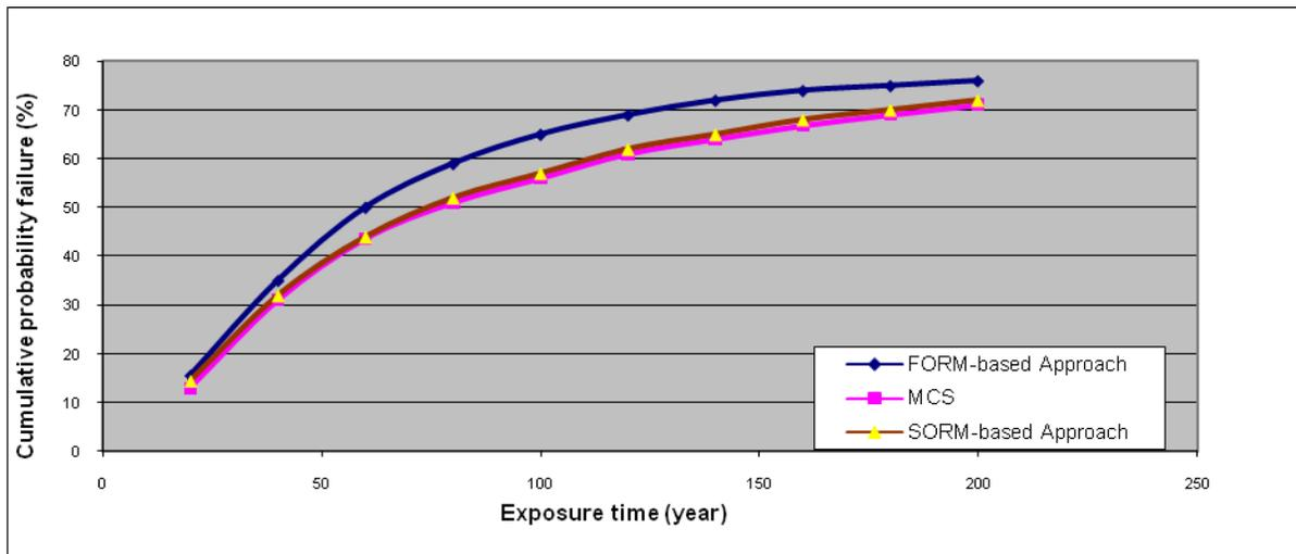
Figure 2.2. Probability of failure throughout the exposure time, for a normal distribution using MCS and FORM- and SORM-based approaches (203 mm pipe diameter and failure criteria of
