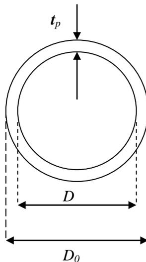
Figure 2.1. Section of a pipe segment with outer and inner diameters
