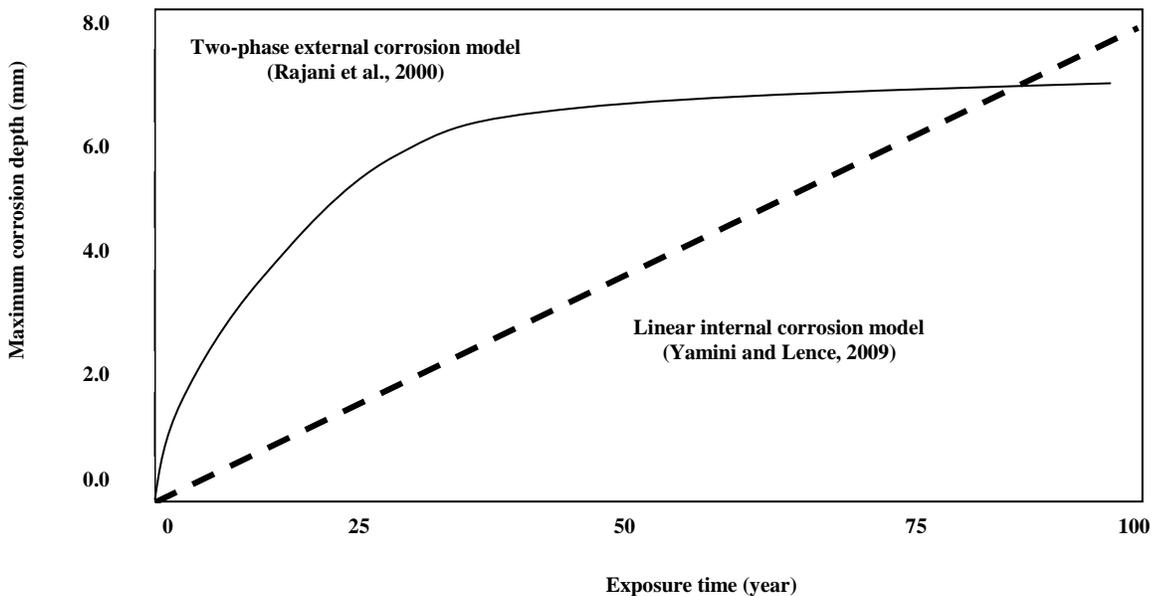
Figure 3.1. Predictive external and internal corrosion models for corrosion depths
