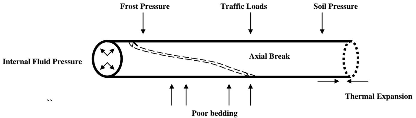
Figure 1.4. Longitudinal failure mode for cast iron pipe
