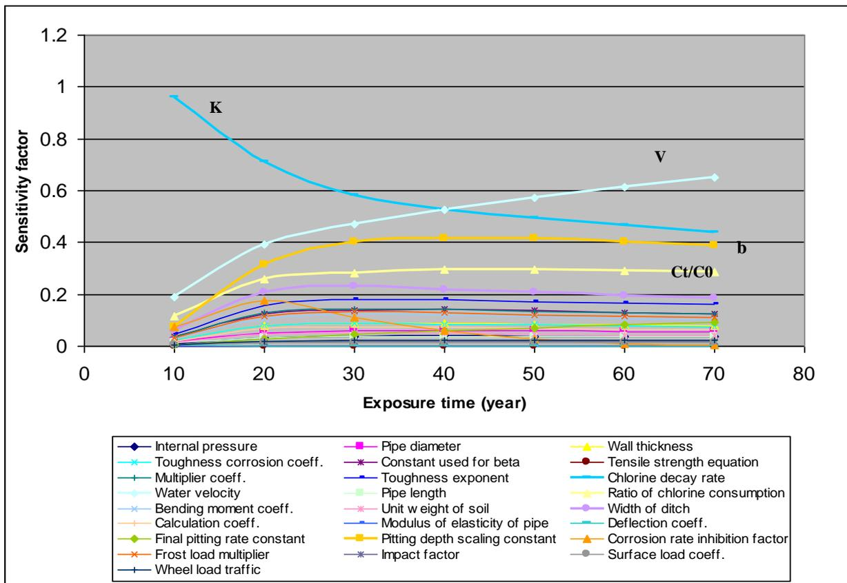
Figure 3.5. Sensitivity factors for input variables throughout the exposure time using a SORM-based approach (external and internal corrosion, failure criteria of  $\sigma_{\theta} \geq \sigma_Y$ )
