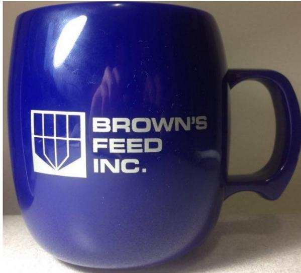
Figure 3: Straight on view of a corn plastic mug that has been put through a home dishwasher 16 times
