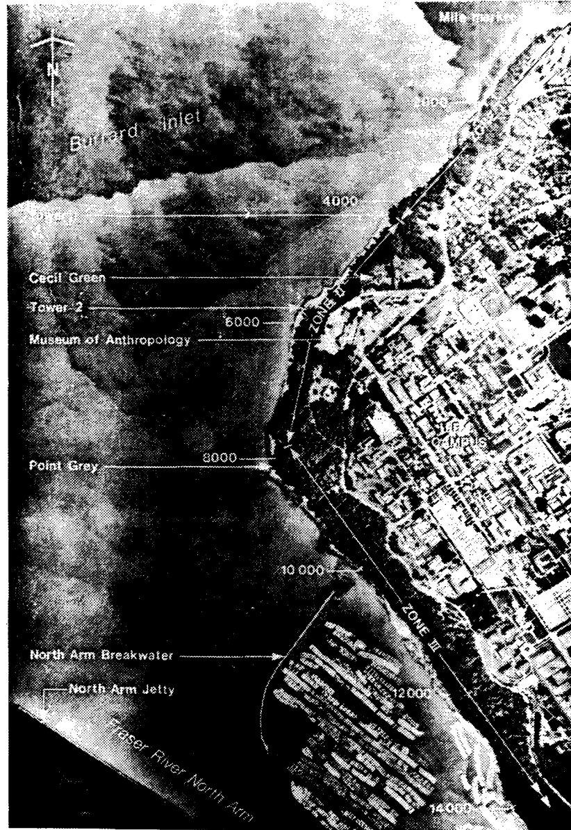
Plan view of Point Grey peninsula shows three zones where erosion control measures should be taken to control cliff erosion. Report prepared for UBC committee proposes only minor work in Zones I and III. Major work is proposed for Zone II between Tower One and geographic point called Point Grey.
