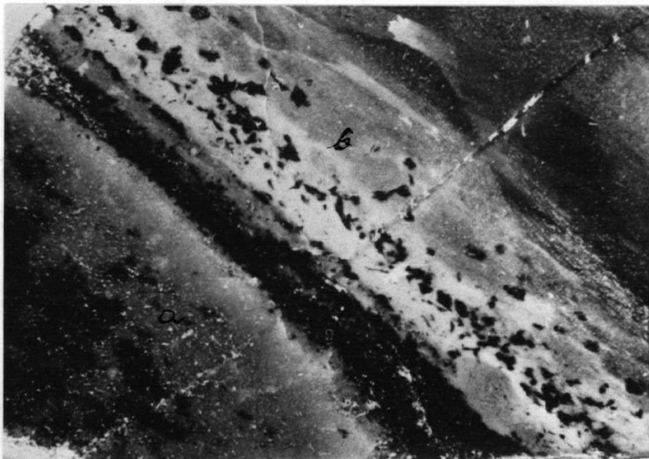
Figure 16. Polished specimen of a zoned boulder. (a = boulder, b = reaction zone; see analyses 3a and 3b on page 53). Note the distribution of biotite (black). The wide biotite band defines the contact between the boulder and the reaction zone.
