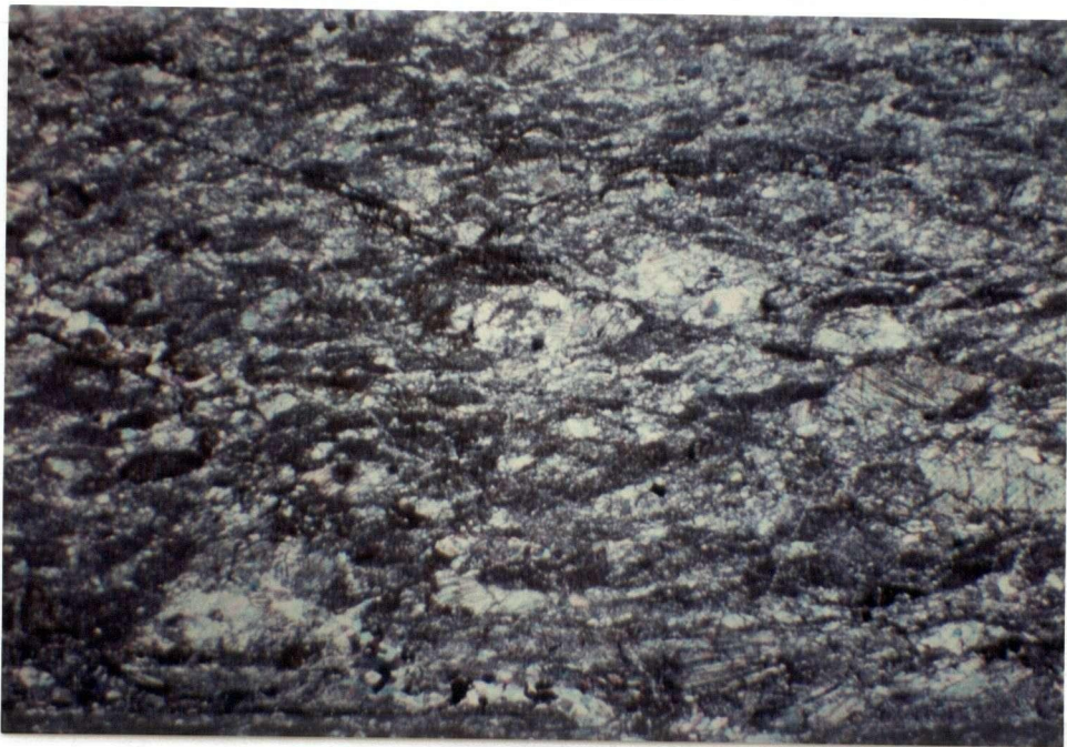
Figure 3.10: Photomicrograph in cross polarized light of flattened oncolites and/or oöliths in carbonates north of Porcupine Creek (NPORCCK-1). Magnification x30.
