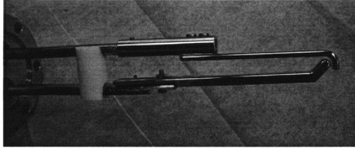
Figure 6.3: A picture of the high DC voltage electrodes attached to a 1.33" vacuum CF flange electrical feedthrough before being inserted in the vacuum chamber. The spacing between the electrodes at the curved end, where the cold atoms would be inserted is around 1.3 mm.
