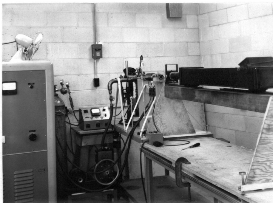
Figure 5. The apparatus assembly of the induction furnace, vacuum system and optical system.
