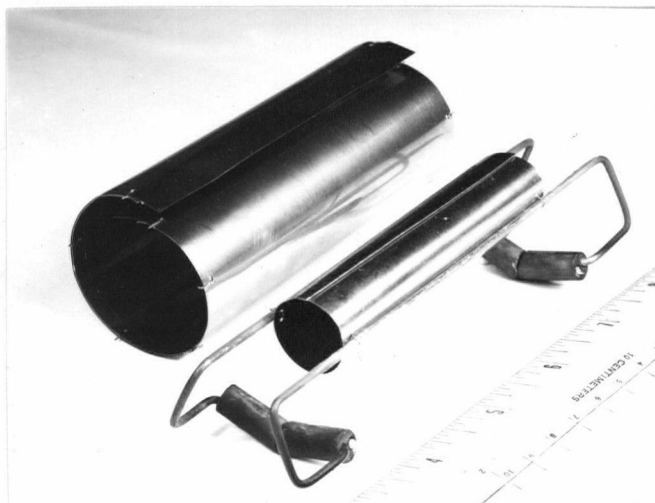
Figure 7. Molybdenum heating elements (dismantled) of the induction furnace.
