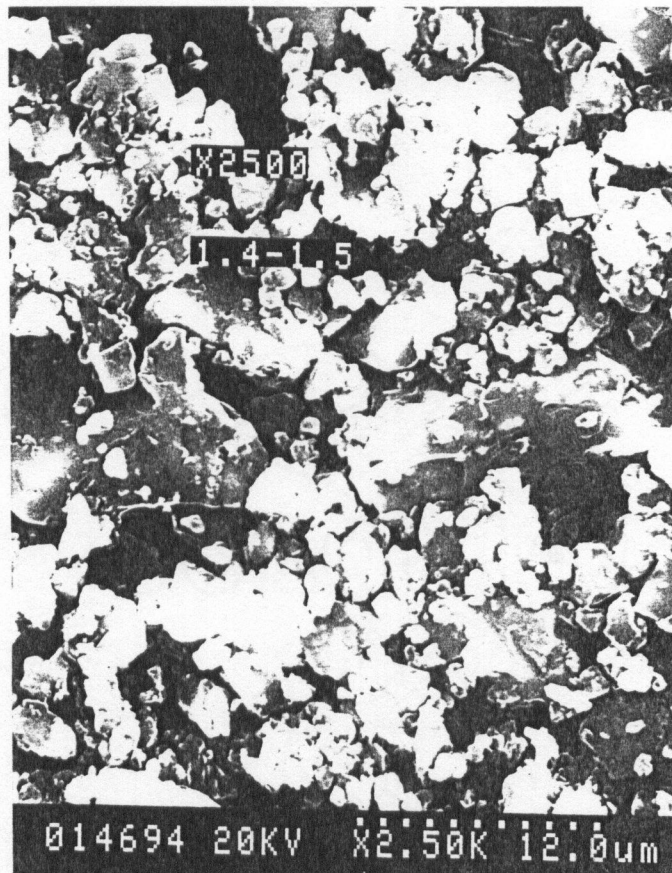
Figure 6.8.2 (b) SEM photograph of the same pellet surface Magnified by 2500 times
