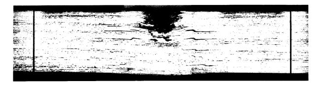
Figure 5.7 Micrographic illustration of delamination initiation in a 6.15 mm thick CFRP specimen when penetrated by an indenter with 37° cone angle (Sanders, 1997). The delaminations are located below the indenter and matrix cracks nearby.
