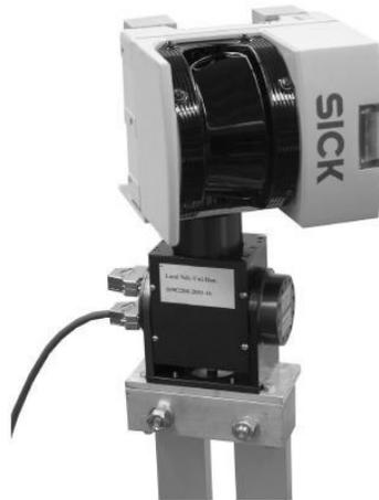
**Figure 1-2.** 3D scanner consisting of a 2D scanner and servo driver
