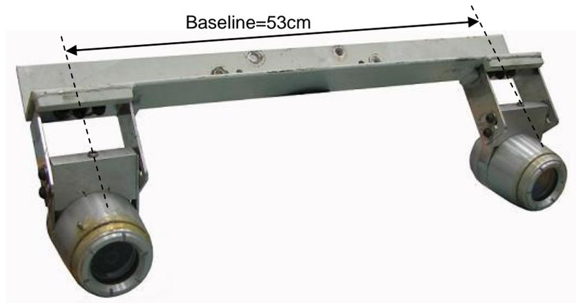
**Figure 2-3.** The designed torso-mounted stereo camera rig (Courtesy of Motion Metrics Int'l)
