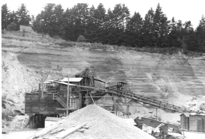
1. Quarrying the Cordova sands and gravels near Cordova Bay. Output of this operation is about 15 yards of washed and sorted materials per hour.
