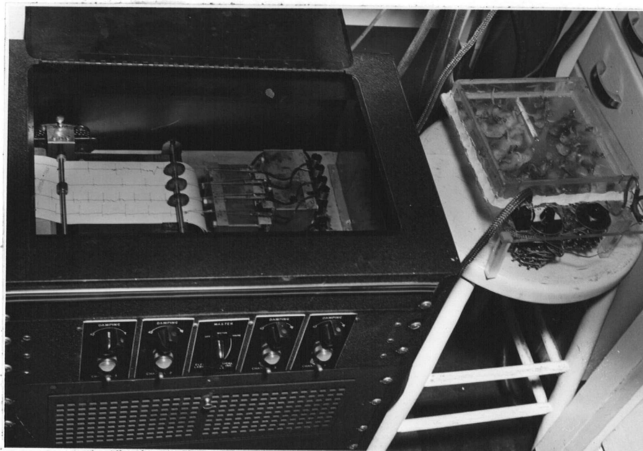
Fig. 7. Recorder Connected to Electrodes Housed in Airtight Plastic Box , showing 11 subjects in the nitrogen chamber. The circuits lead through the respective amplifiers and terminate in the four direct-writing galvanometers, photographed in the process of tracing electrocardiographic patterns.
