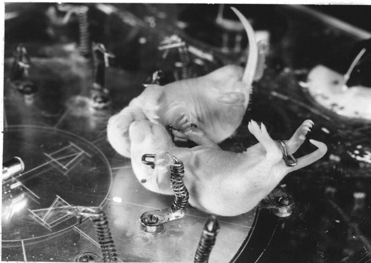
Fig. 5. Detail of Electrodes and Immobilization of Subjects, showing the design of the nickel-silver clips which, attached to the right foreleg and left hindleg of each subject, immobilized the animal and carried to the recorder-amplifier the Standard Limb Lead II of the Electrocardiogram.
