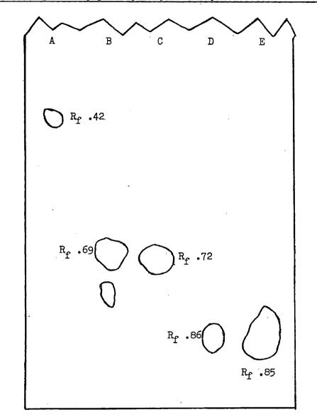
Chromatogram of pepsin hydrolysis of synthetic substrates
