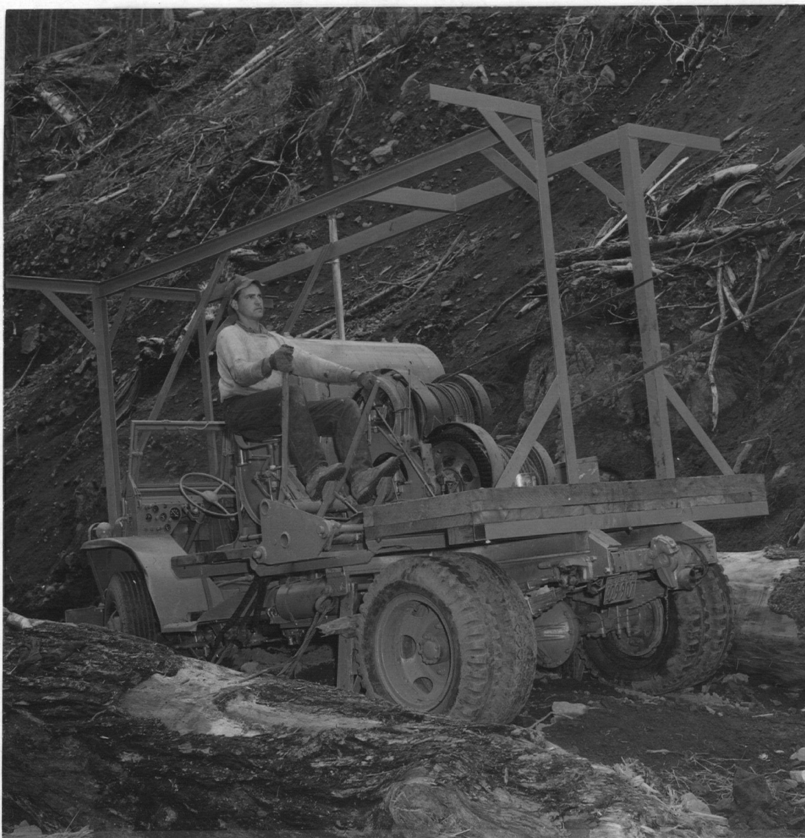
Fig. 3. Truck-mounted Skagit B.U. 15. Used for yarding salvage with conventional spar.
