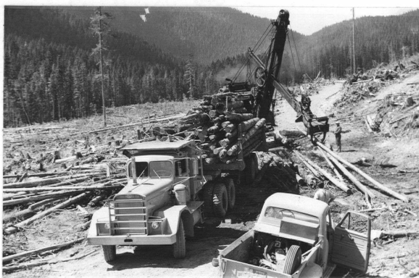
Fig. 15. Shovel with Berger air-tongs loading salvage logs.
