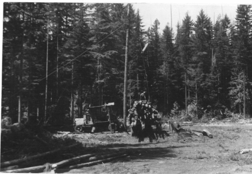
Fig. 20. Prepared bundles being loaded onto a truck. Gin pole loader.
