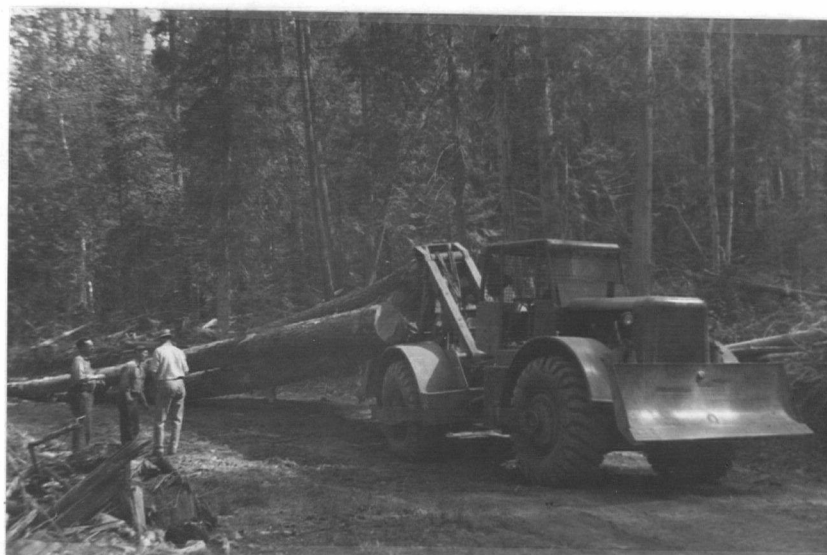
Fig. 41. Wagner TRD 14. Loggermobile. Skidding tree length logs.
