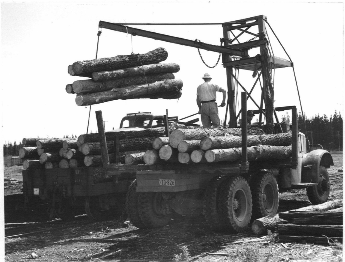
Fig. 13. Crane truck for yarding, loading, transportation and unloading logs.
