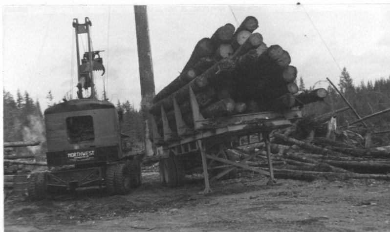
Fig. 23. Maxi-mounted Northwest loading salvage onto salvage trailer.
