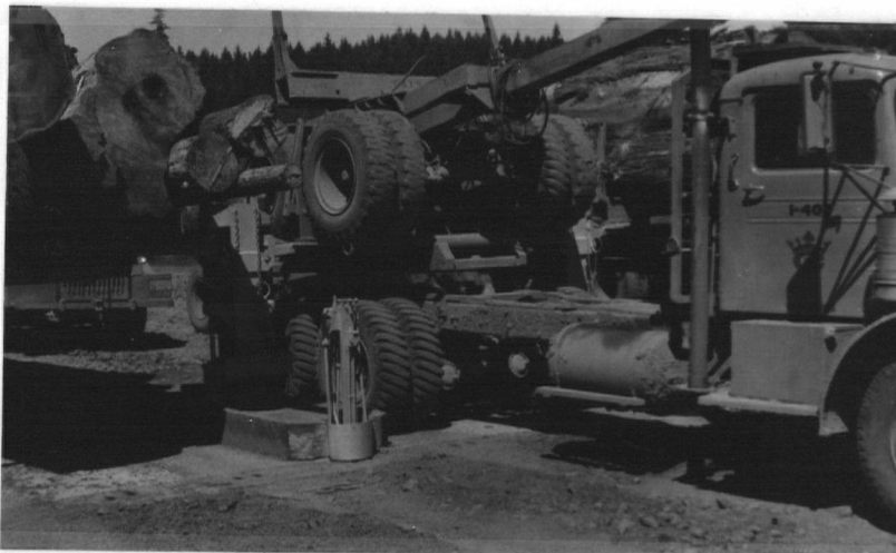
Fig. 46. Close up of transfer point at Columbia Tree Farm to show hydraulic cylinders at base of stanchion.
