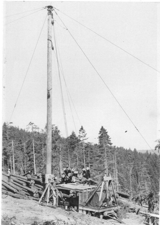
Fig. 6. 70' mobile spar and B.U.30 Skagit yarder mounted on disused transporter.
