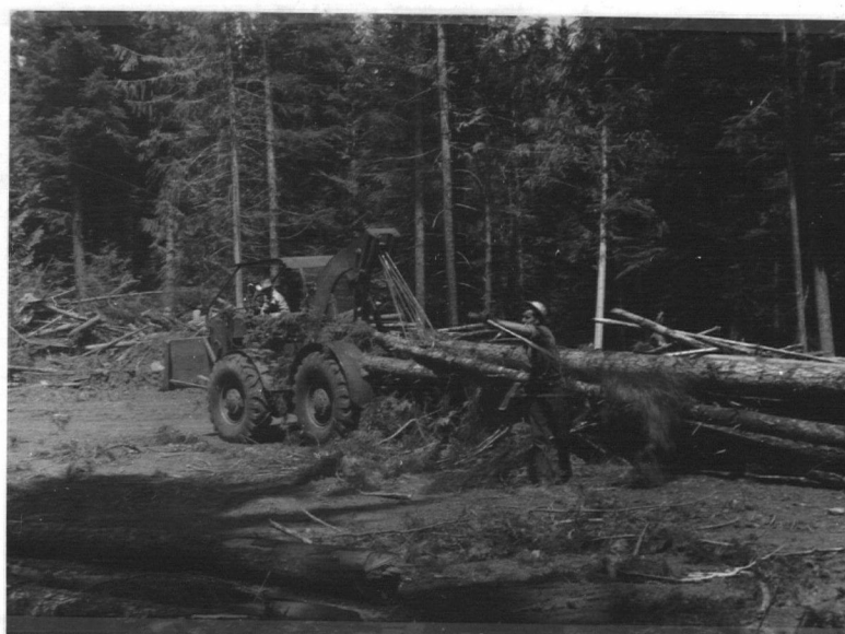
Fig. 31. Westfall "100" rubber tired tractor skidding thinnings.
