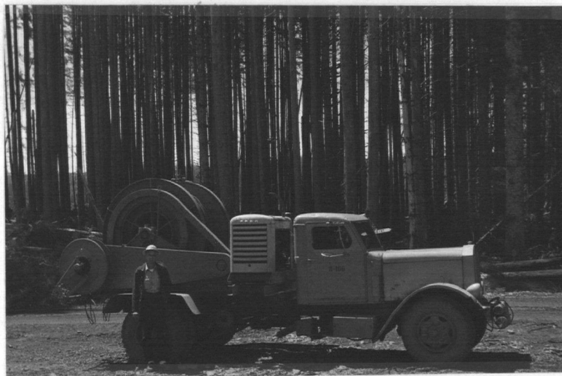
Fig. 52. Guyline pick-up drum and rig-up goat on out of date truck.
