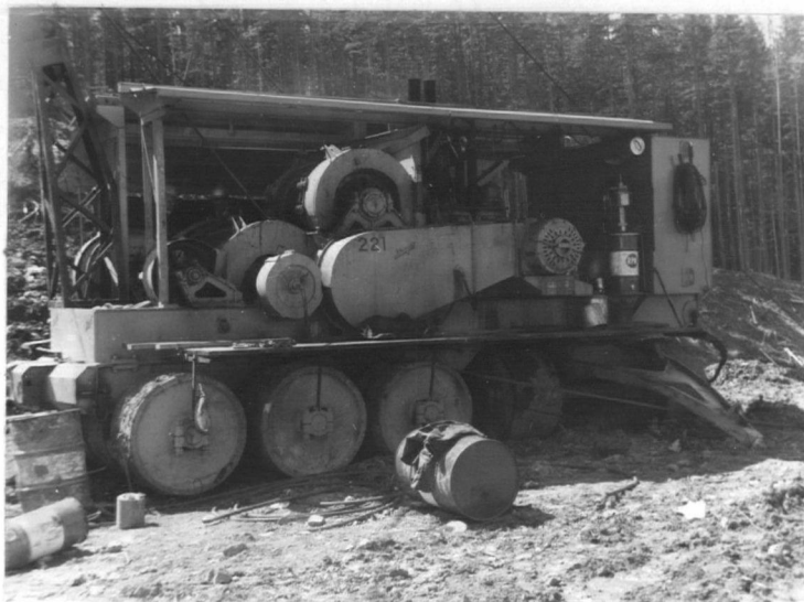
Fig. 48. Solid steel wheel chassis for large Skagit yarder. Moved by D.8.
