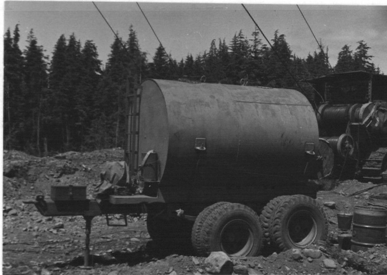
Fig. 51. 600 gallon water tank on old logging-trailer.
