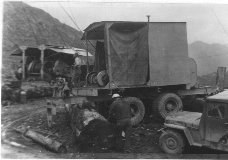
Fig. 50. B.U.15 Skagit loader mounted on disused truck-chassis.
