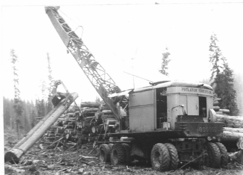
Fig. 53. Maxi-mounted Osgood loading crane.
