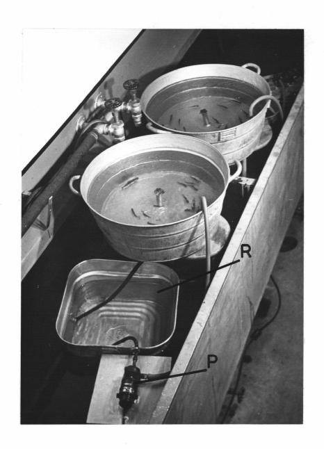
Figure 4. Rheotaxis tubs with kamloops trout orienting in circular currents. R, reservoir surrounded by water to control temperature; P, Eastern centrifugal pump.
