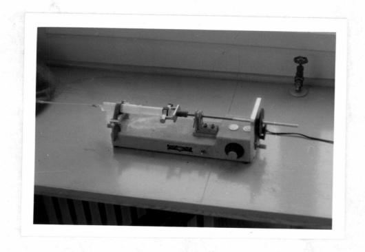
Figure 2. Continuous delivery infusion machine.
