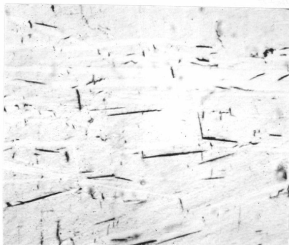
Figure 20 Same held at 700°C for 24 hrs. after 1 hr. at 900°C. Transformed \beta . Etch No. 2 x 800.
