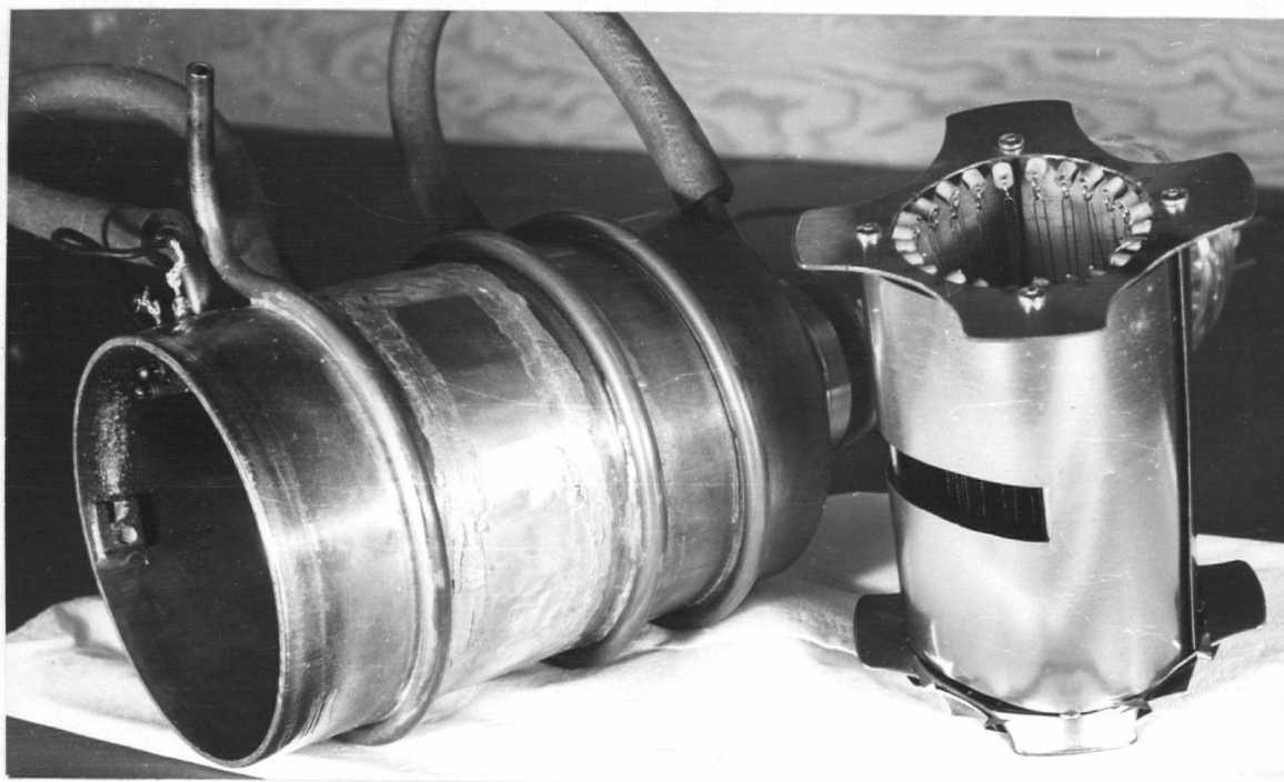
Figure 9. High-temperature x-ray unit furnace with a zirconium radiation shield and the external, water-cooled can.
