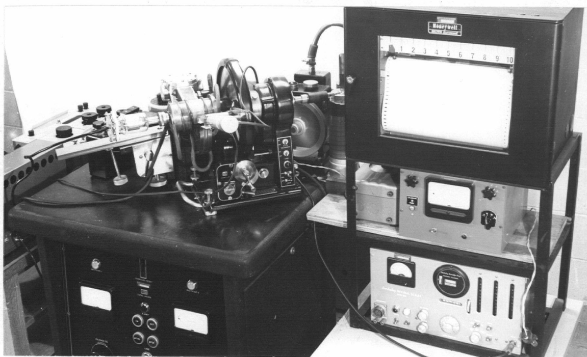
Figure 12. View of high-temperature x-ray unit showing the Geiger-counter scaler, rate meter and recorder.
