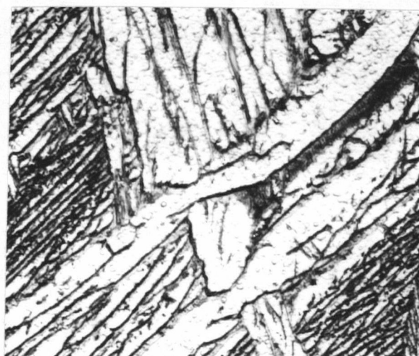
Figure 16 Same equilibrated to 450°C. \alpha . Etch No. 2 x 800.
