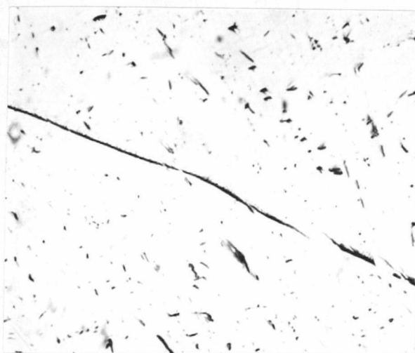
Figure 15 85.4% Zr-10.3% Ti-4.3% Nb as-cast. Transformed \beta , i.e., \alpha' . Chemical polish No. 1. Etch No. 1 x 800
