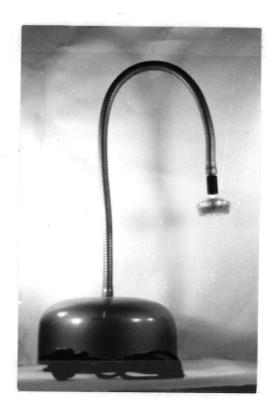
PLATE III. Photograph of a tritium ion generator. (Used in the production of negatively ionized air).
