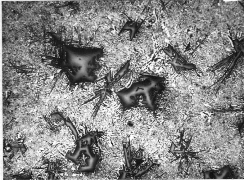
Figure 15. Alloy No. 1 unrefined. 0.5% HF etch
