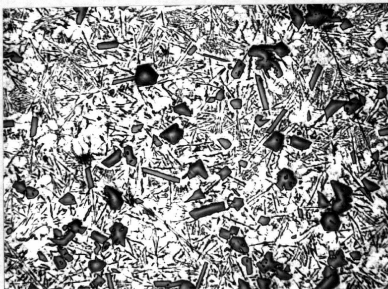
Figure 19. Alloy No. 7 refined by 0.32% P added as \text{PCl}_5 . Cast 5 minutes after \text{PCl}_5 added. 0.5% HF etch. 150x
