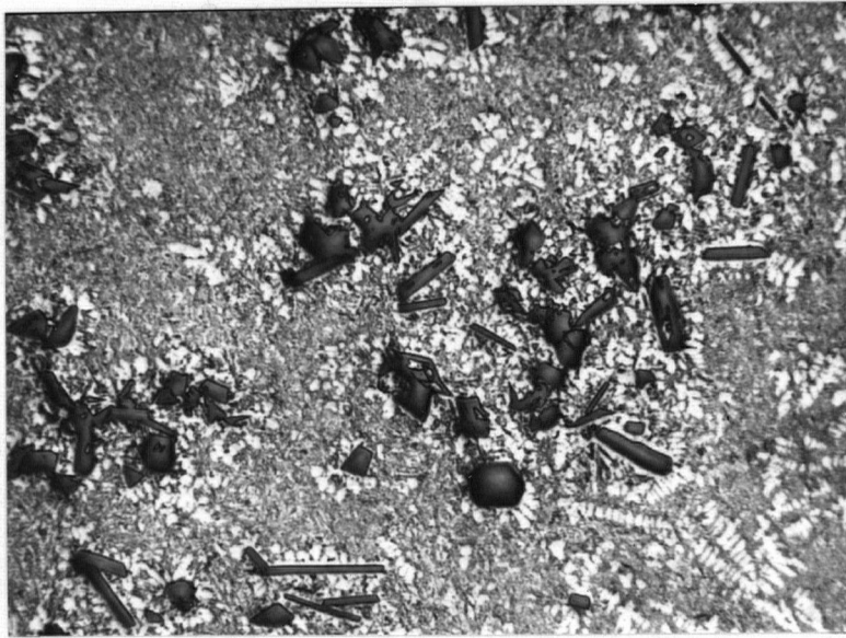
Figure 29. Alloy No. 11 containing 0.5% magnesium and 0.2% phosphorus, 0.5% HF etch. 150x
