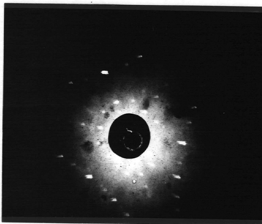
Figure 31. Specimen of Figure 30 rotated 35.3^{\circ} towards [001] . Note the 3-fold symmetry of the [111] direction.
