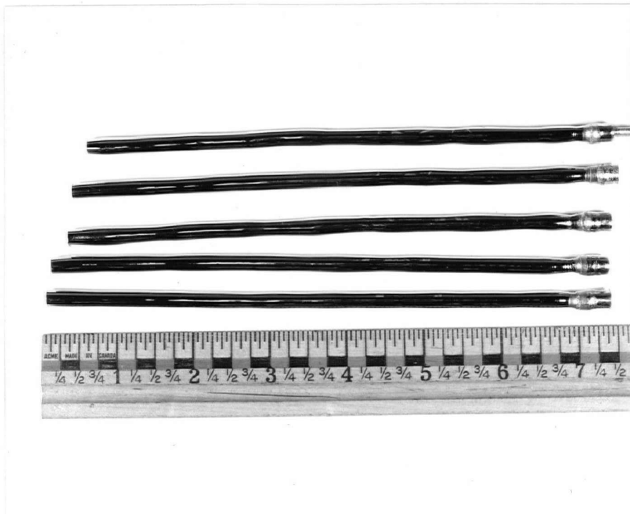
Figure 7. Photograph of Vanadium Single Crystals Grown by the Melt-Solidification-Zone-Refining Technique
