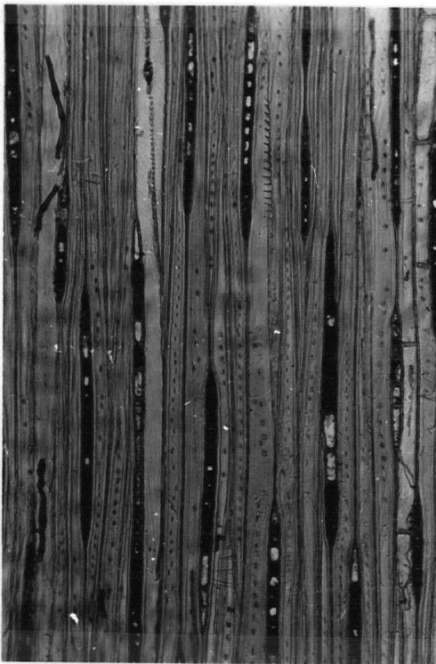
Fig. 18. Beilschmiedia erythrophloia Hay. (x-sec., t-sec. and r-sec.) at 100 x
