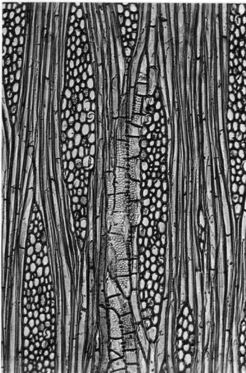
Fig. 35. Tectona grandis Linn. f. (x-sec., t-sec. and r-sec.) at 100 x
