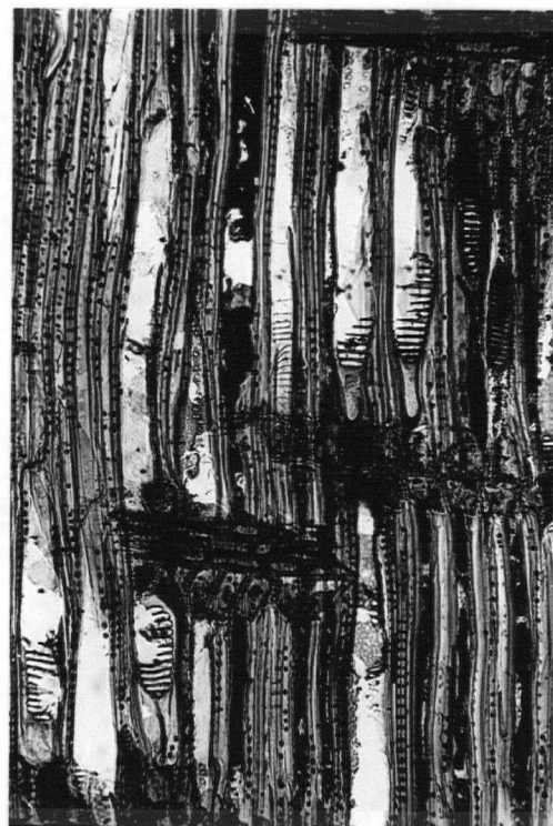
Fig. 29. Gordonia axillaris (Don.) Szysz. (x-sec., t-sec. and r-sec.) at 100 x
