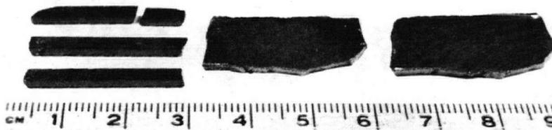
Figure 5 Slabs and rough-cut specimens of fused uranium dioxide
