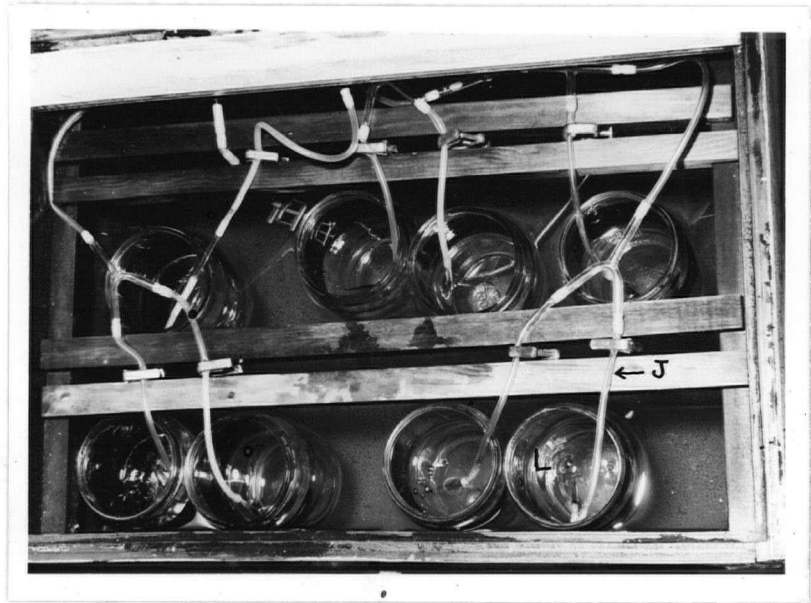
Figure 3. Arrangement of bottles in a tank for experiments XI - XIV. J - Air jet; L - Bottle.
