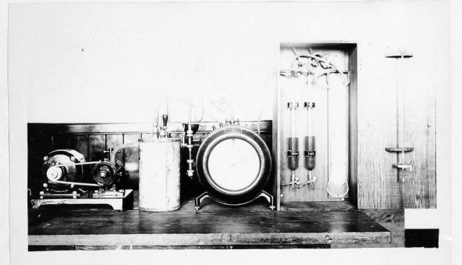
The absorbers contain 100 c.c. of an iodinepotassium iodide-starch solution about 0.00003 N in iodine. Through one absorber containing this solution a metered volume of air is drawn as a "blank" using a soda-lime tower. Through the other absorber the same volume of air is drawn from the
