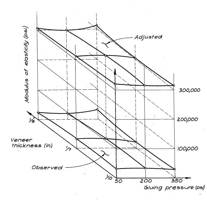
Figure 7. Influence of controlled factors on modulus of elasticity of sawn-veneer blocks in tension.
