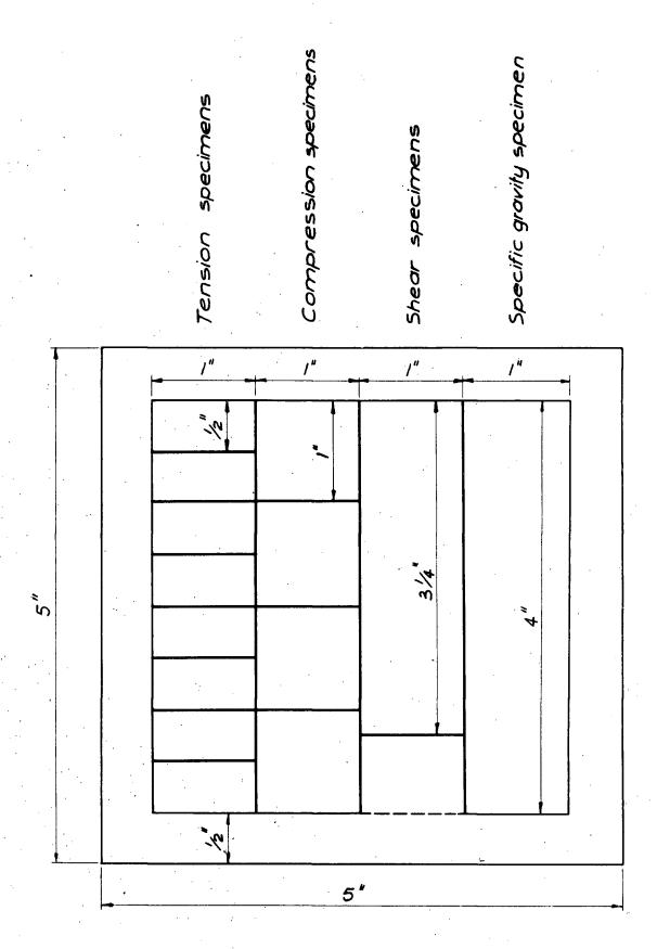
Figure 1. Cutting plan of plywood blocks.
