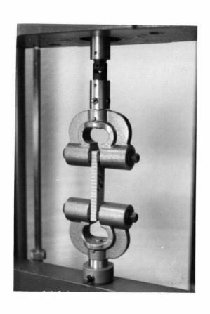
Figure 5. Tension specimen in the grips of the table model Instron testing instrument.
