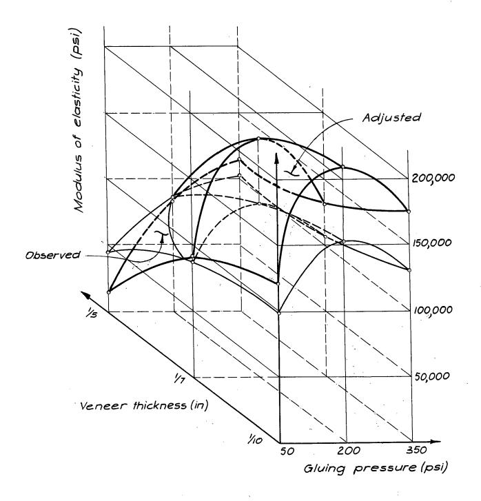
Figure 8. Influence of controlled factors on modulus of elasticity of rotary - cut veneer blocks in compression.
