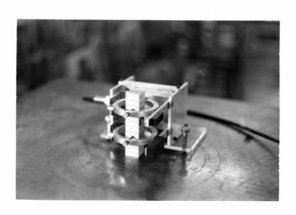
Figure 3. Compression specimen in the microformer extensometer.
