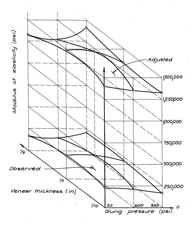
Figure 6. Influence of controlled factors on modulus of clasticity of sawn-veneer blocks in compression.
