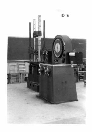
Figure 2. Baldwin Universal Testing Machine in the materials testing laboratory of the Faculty of Applied Science.
