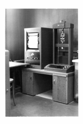
Figure 4. Table Model Instron Testing Instrument in the wood technology laboratory of the Faculty of Forestry.
