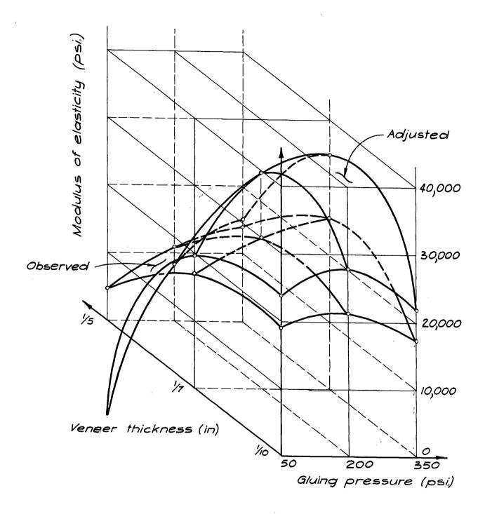
Figure 9. Influence of controlled factors on modulus of elasticity of rotary - cut veneer blocks in tension.
