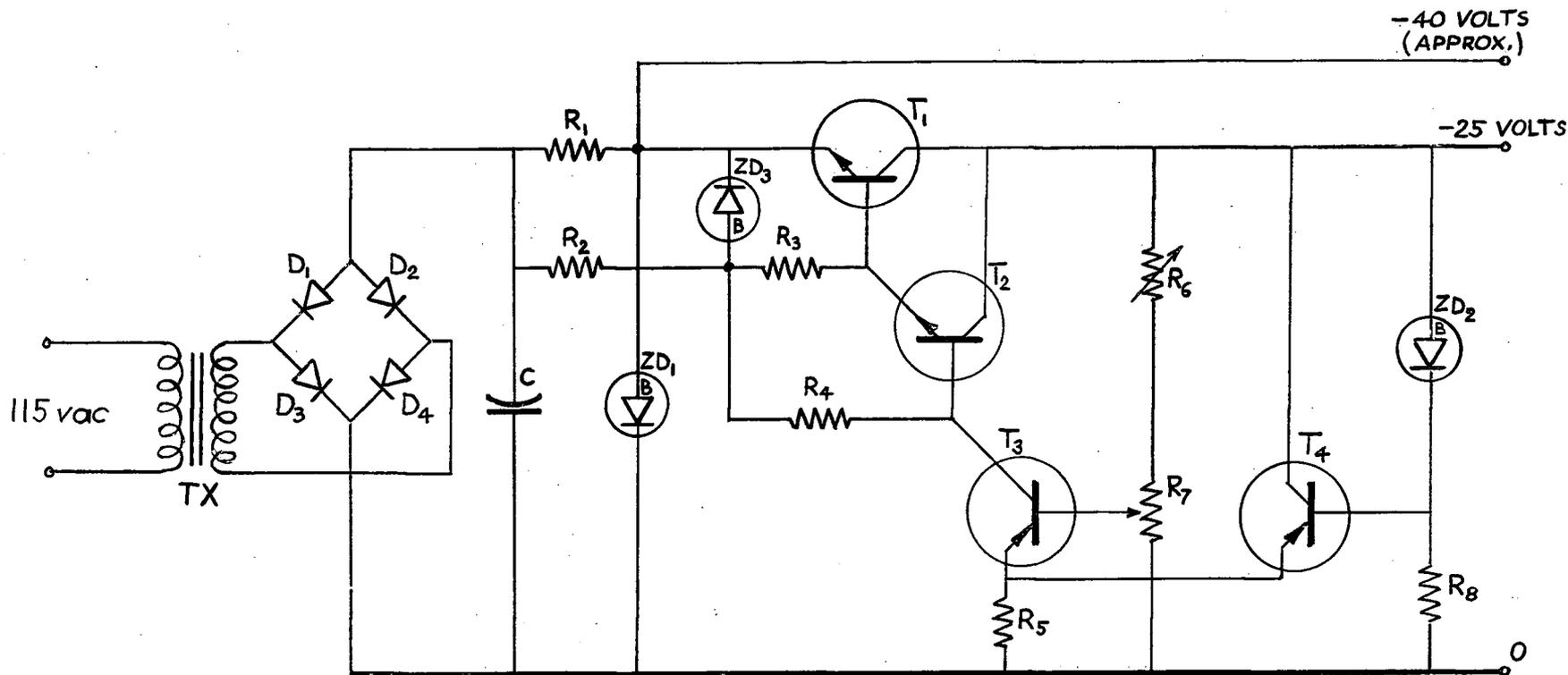
Fig. 19. Short-Circuit Proof Regulated Power Supply
