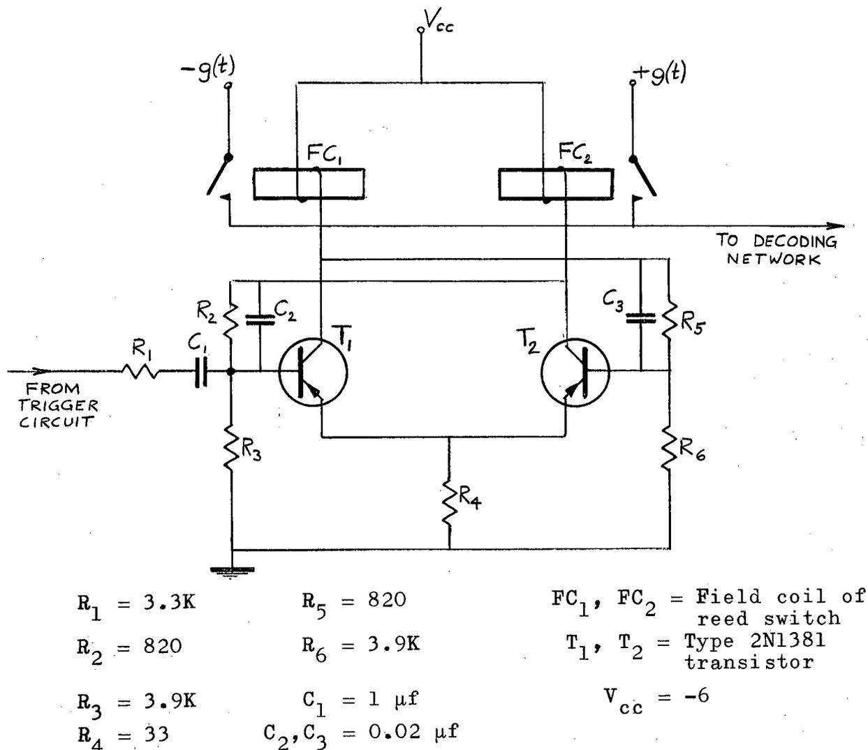
Fig. 16. Switching Circuit for Channel B
