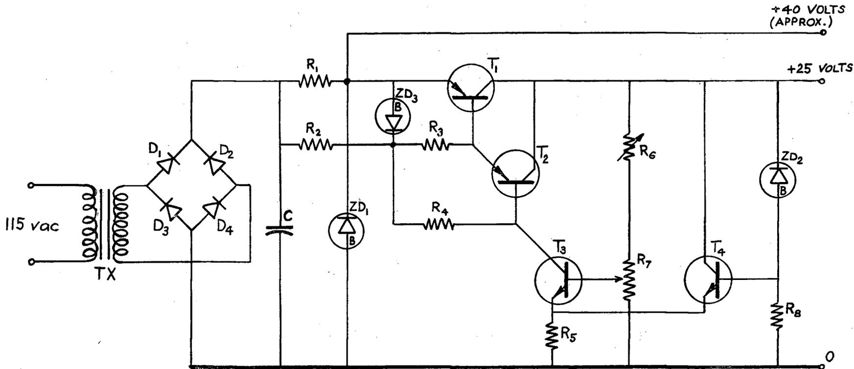
Fig. 20. Short-Circuit Proof Regulated Power Supply
