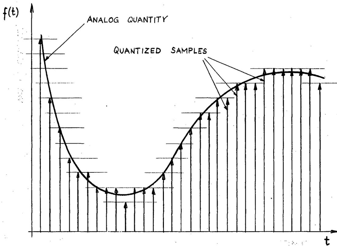
Fig. 1. Digital Representation of an Analog Quantity
