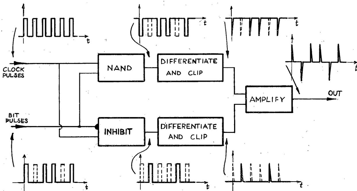
Fig. 11. Generation of Trigger Pulses
