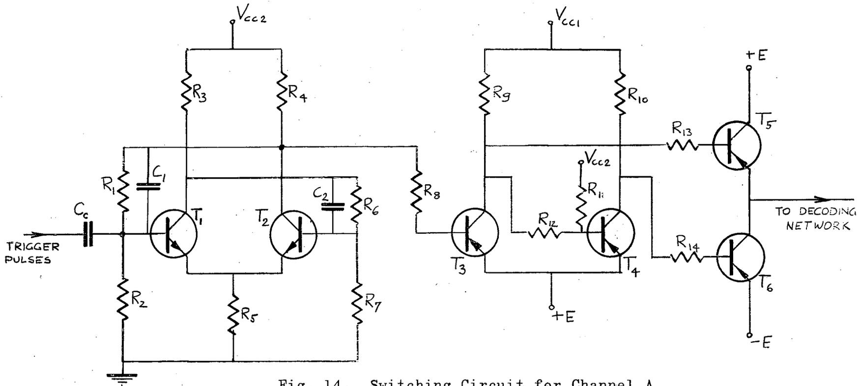
Fig. 14. Switching Circuit for Channel A
