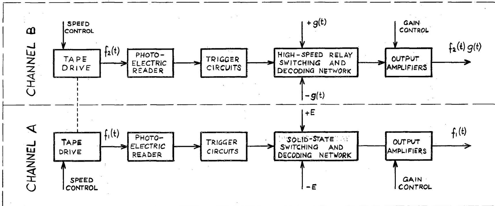
Fig. 8. Block Diagram of the Combination Function Generator and Multiplier
