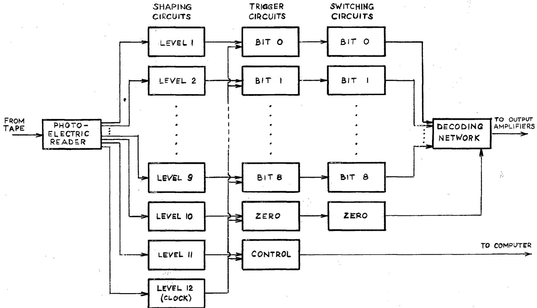
Fig. 9. Details of Tape Level Allocation
