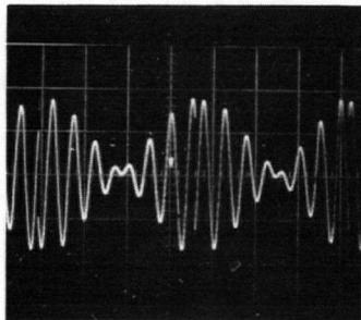
c) Product of the test function and an external function (sinusoidal)
