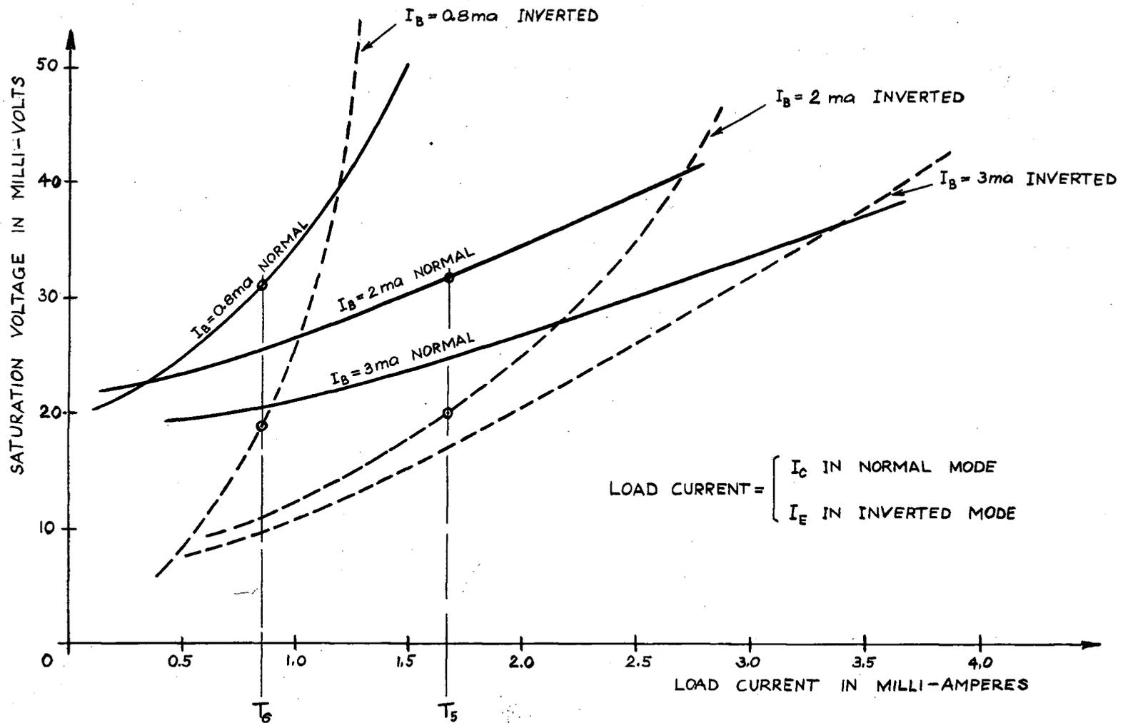
Fig. 15. Saturation Characteristics for the Type 2N398B Transistor
