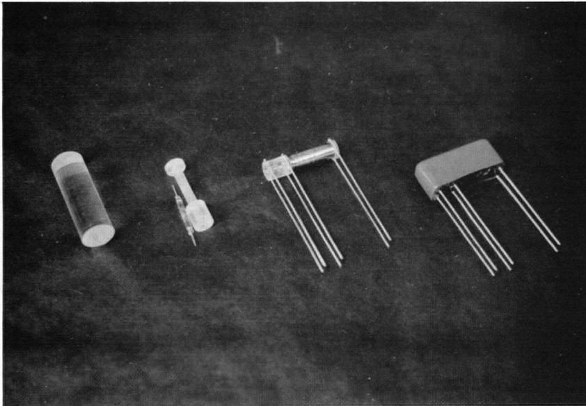
Fig. 28. Construction Phases of the Magnetic Reed Switching Unit
