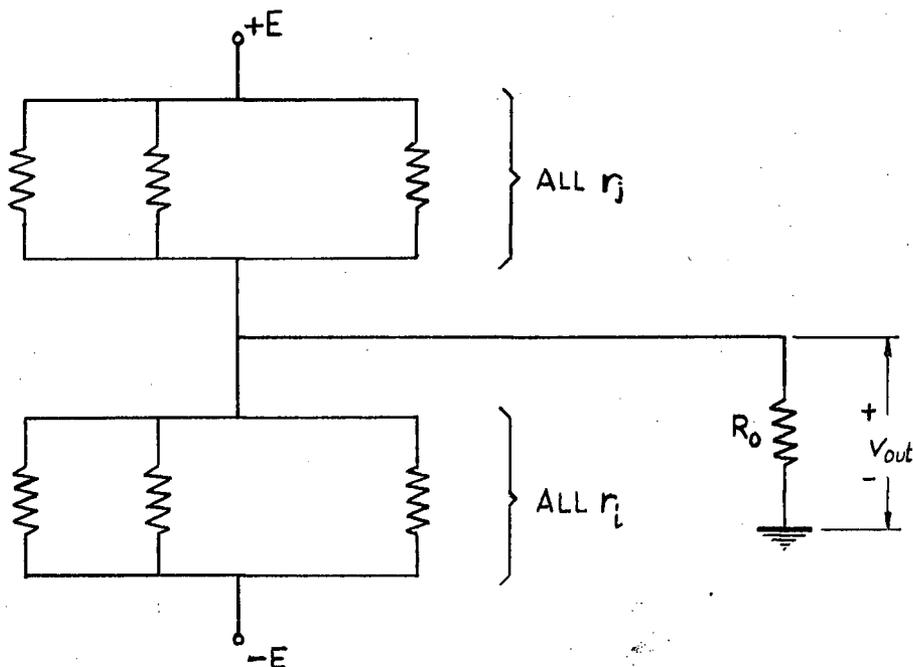
Fig. 4. Equivalent Circuit of the Network of Weighted Resistors
