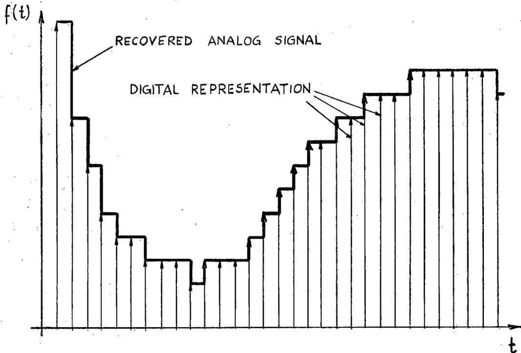
Fig. 2. Analog Signal Recovered from Digital Information
