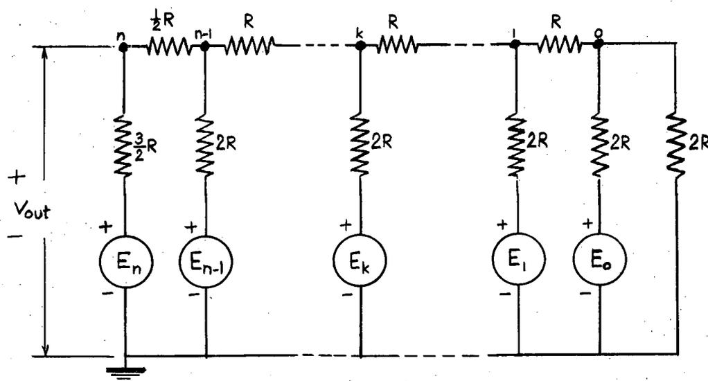
Fig. 5. Ladder Network for Binary Decoding
