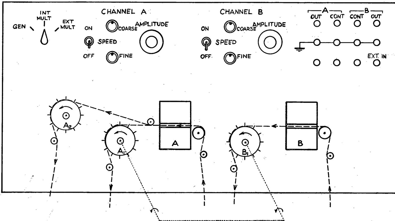
Fig. 22. Control Panel with Tape Drivers
