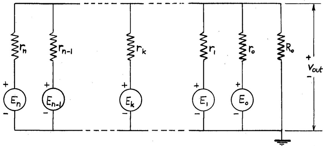
Fig. 3. Network of Weighted Resistors
