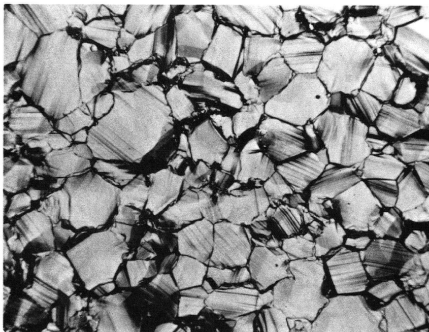
Fig. 26 Lack of twinning in the presence of boundary migration. ( 25 \mu cadmium deformed 10% at +60°C.)
