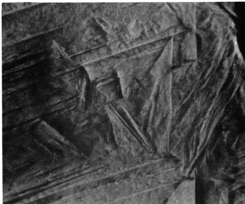
Fig. 13. Fe - 10.79% Ni. Martensite Surface Shears. 1060 X.
