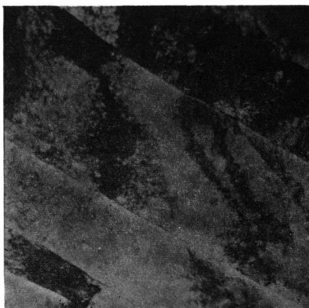
Fig. 4. Pure Iron. Martensite Substructure. 29000 X.
