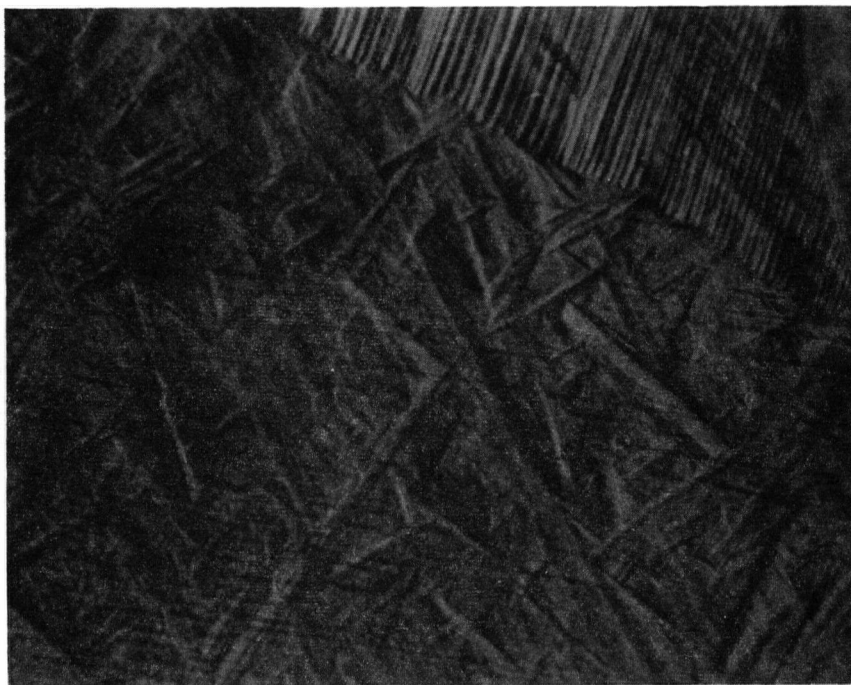
Fig. 3. Pure Iron. Martensite Surface Shears. 1060 X.
