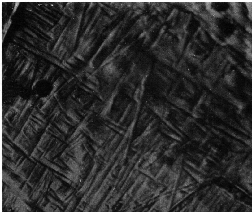
Fig. 9. Fe - 6.0% Mn. Martensite Surface Shears. 1100 X.
