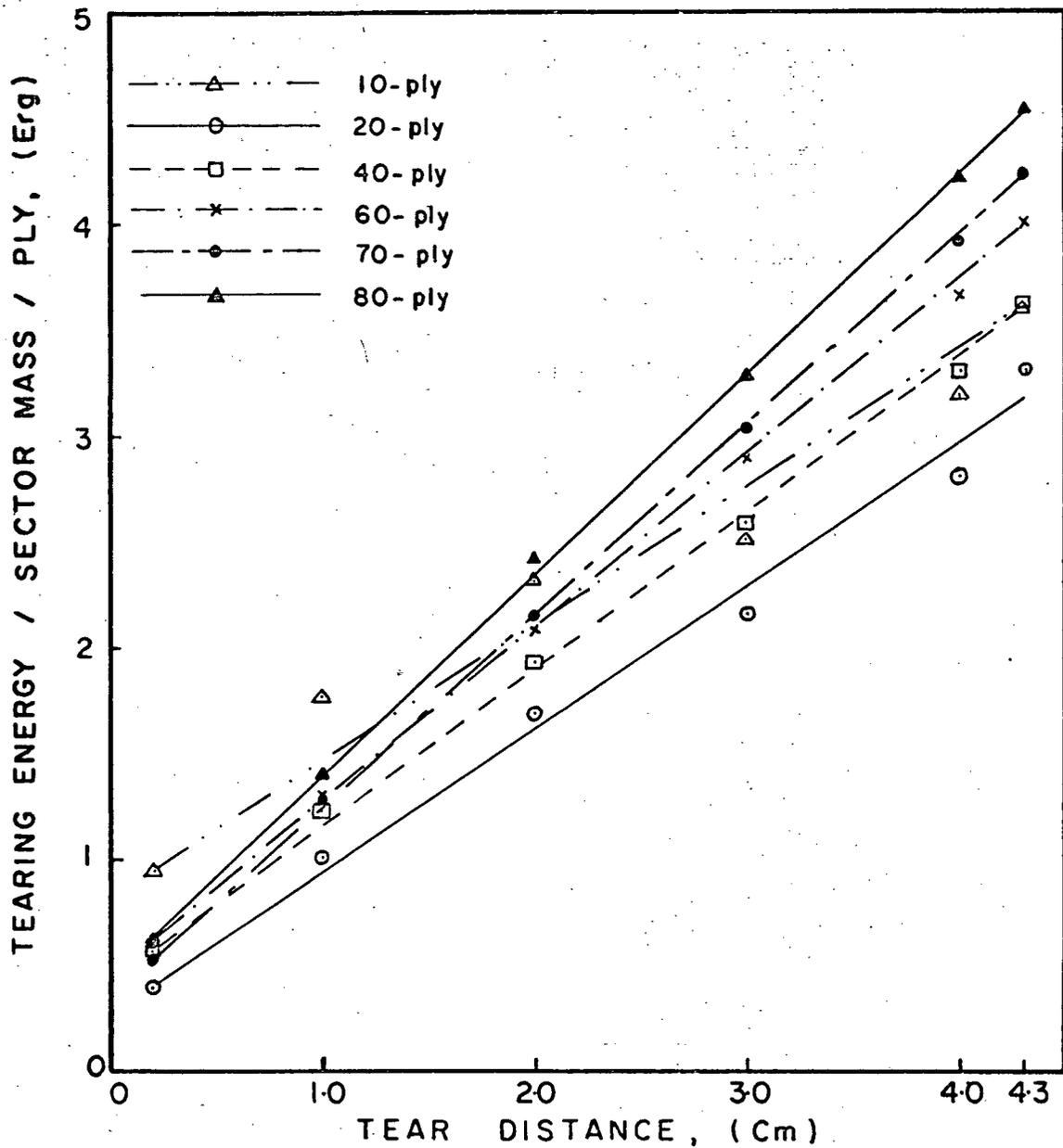
Fig. 15. Relationships between tearing acceleration and number of plies torn simultaneously for five paper grades.
