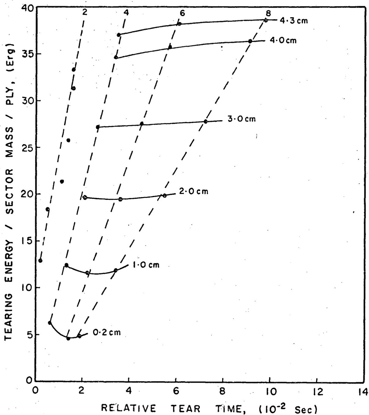
Fig. 11e. Tearing energy, distance and time relationships for parcel wrap. Broken and solid lines are number of paper plies and tear distances, respectively.
