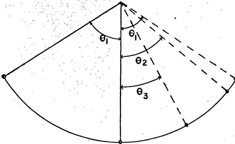
Angles are defined by the vertical line and the line connecting the sector center of mass and axis of rotation.
