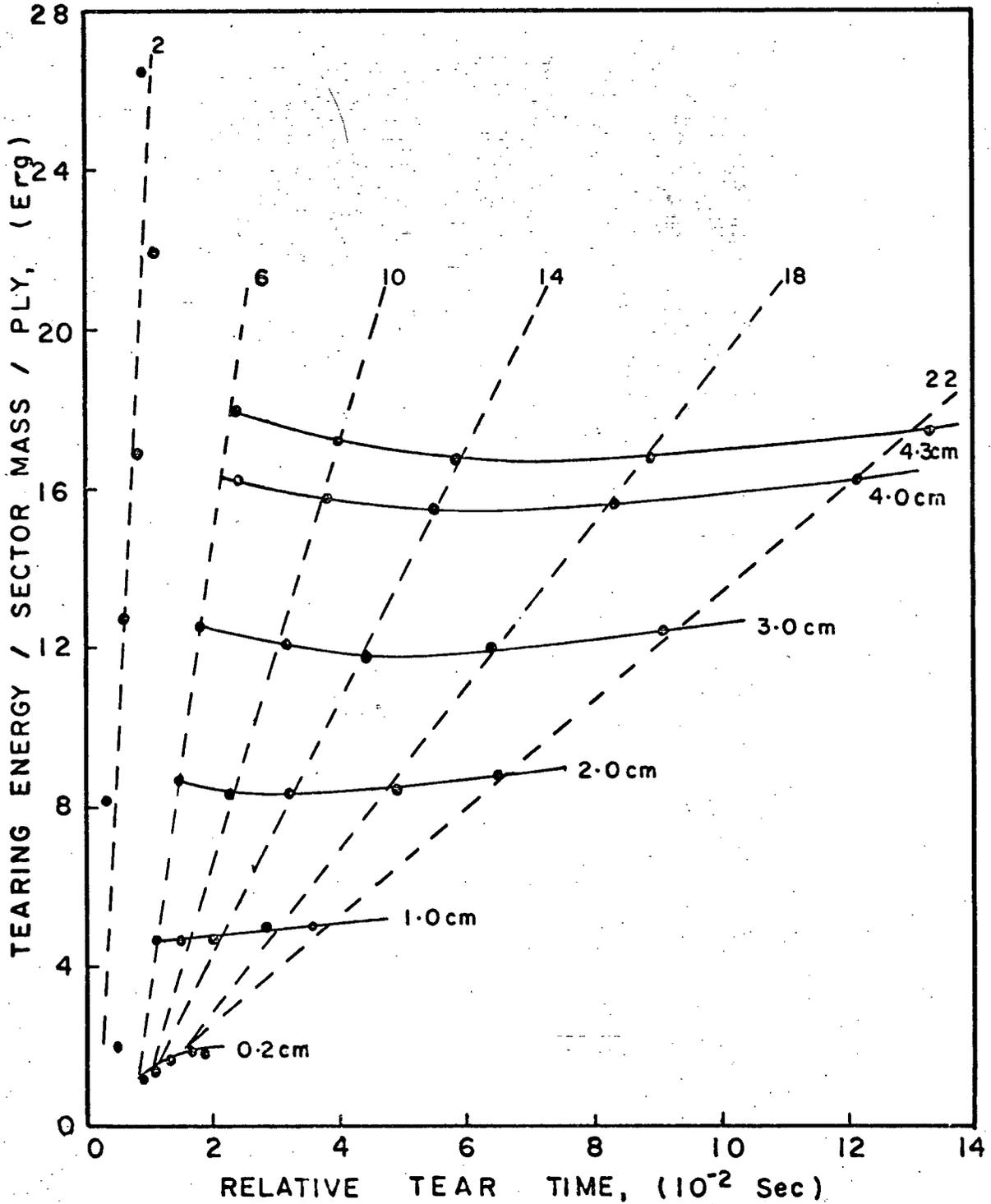
Fig. 1ld. Tearing energy, distance and time relationships for Island 55.5-lb. wrapper. Broken and solid lines are number of paper plies and tear distances, respectively.
