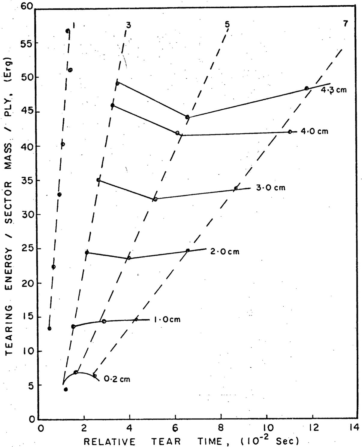
Fig. 12. Relationships between relative tear time per unit ply and number of plies torn simultaneously.
