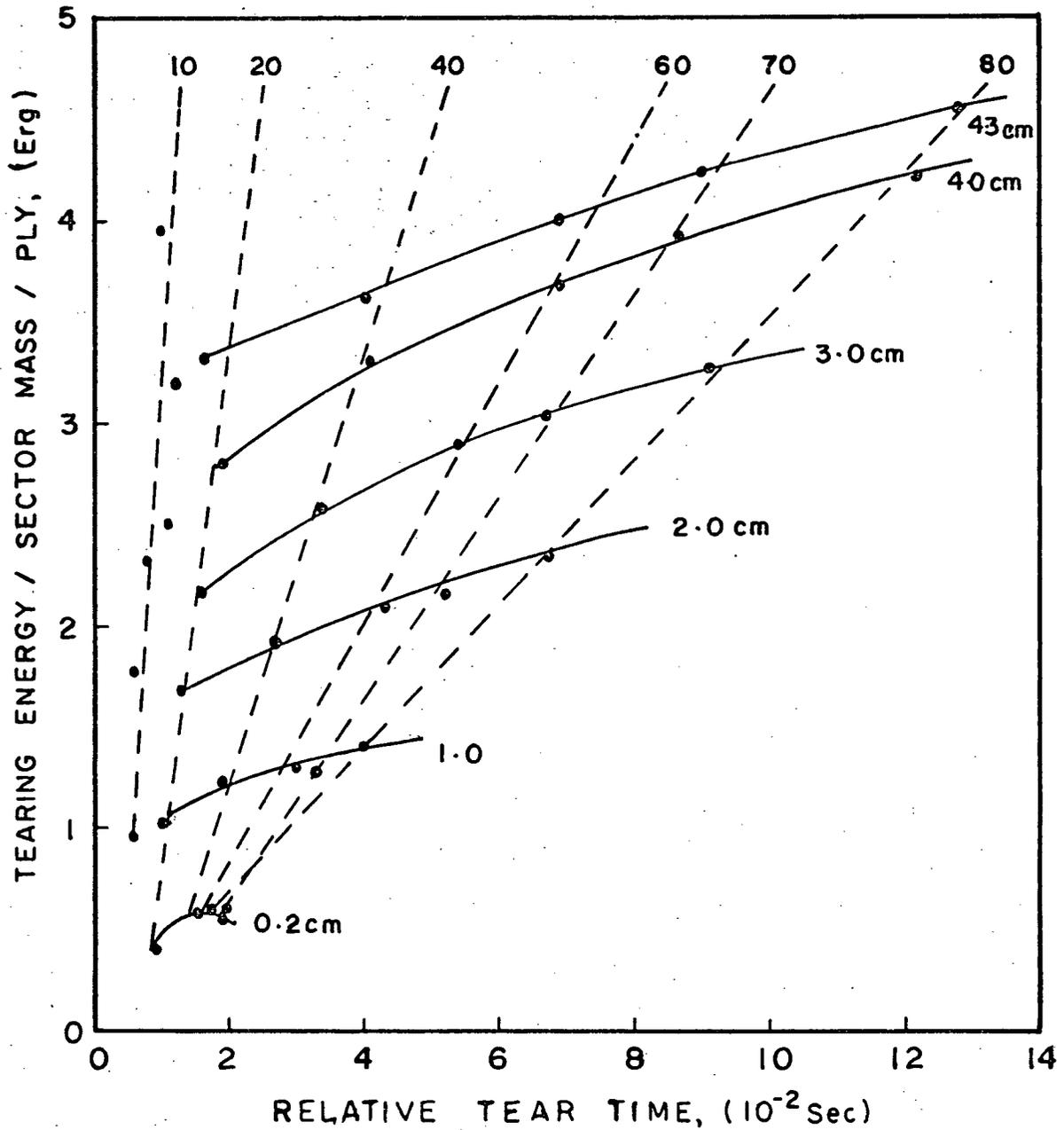
Fig. 11b. Tearing energy, distance and time relationships for newsprint. Broken and solid lines are number of paper plies and tear distances, respectively.
