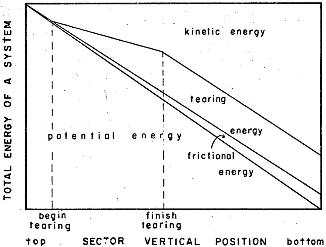
Fig. 4. Schematic diagrams illustrating the conversion of energies in, a. sector swing without specimen, b. sector swing when tearing a specimen.
