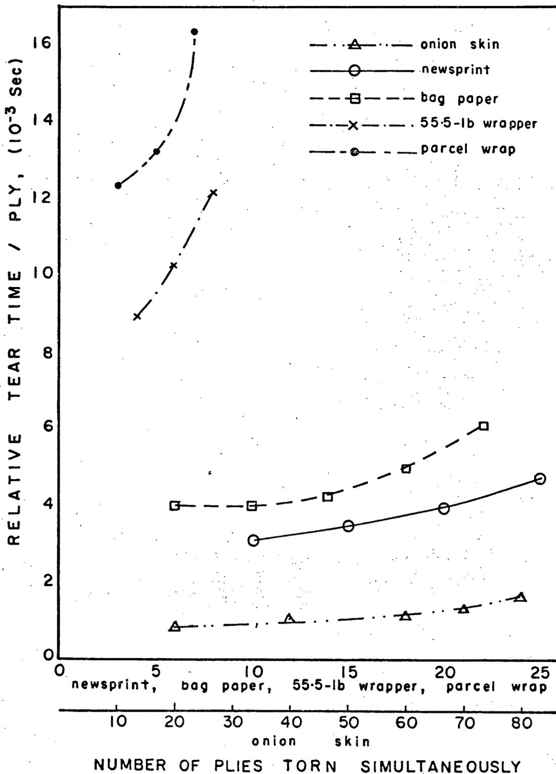
Fig. 13. Relationships between tearing strength and tearing energy for five paper grades.
