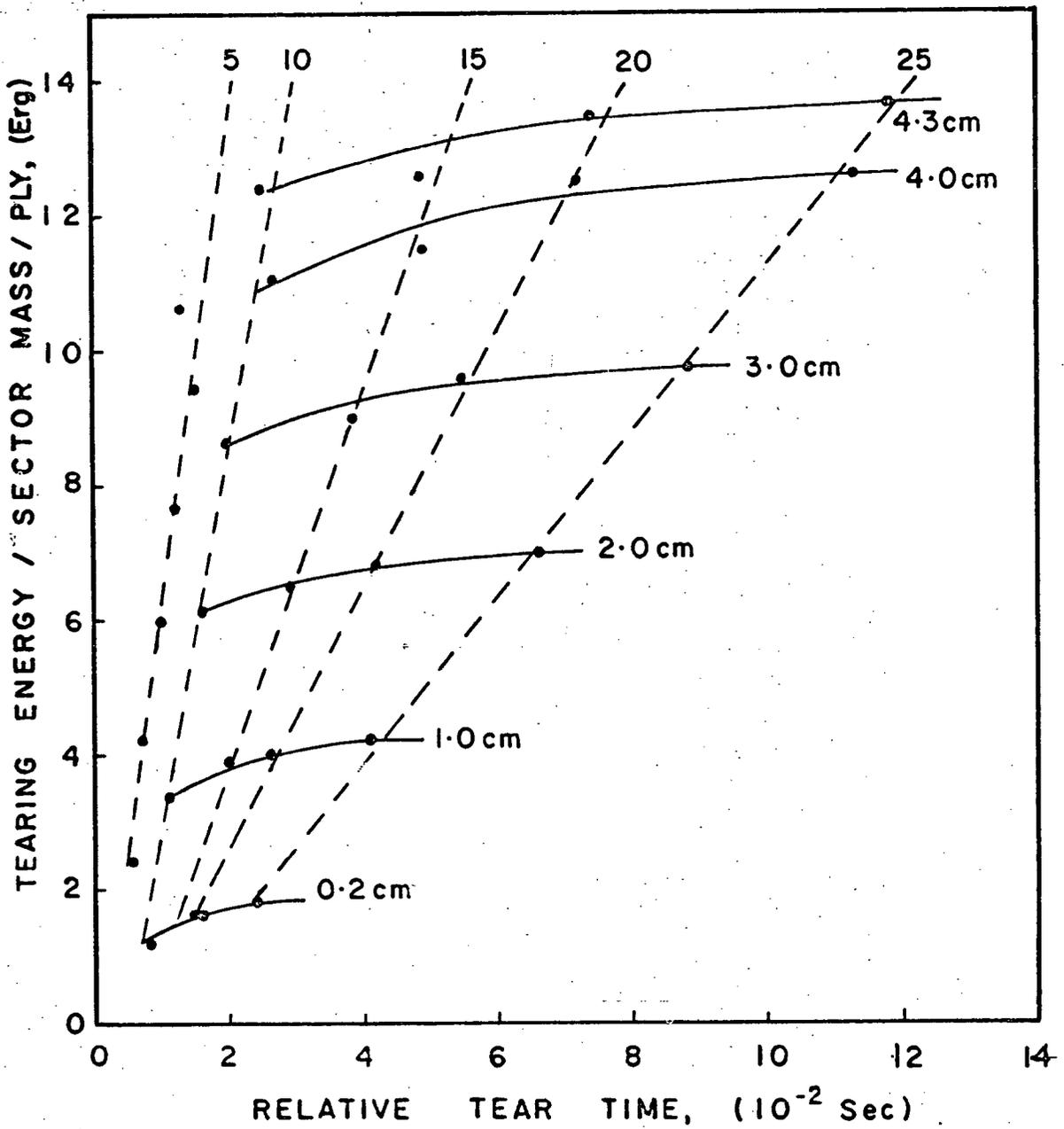
Fig. 11c. Tearing energy, distance and time relationships for 30-lb. n & m bag paper. Broken and solid lines are number of paper plies and tear distances, respectively.
