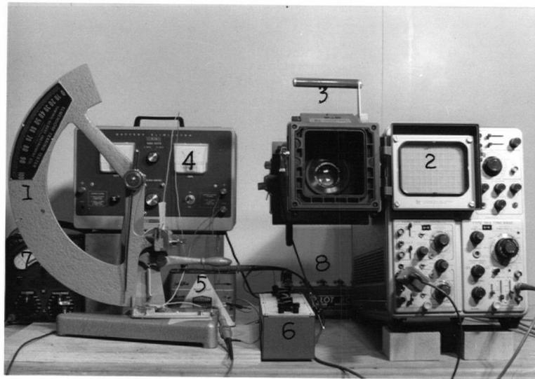
1. Thwing-Albert Instrument Co. No. 60-100 Elmendorf tearing tester.
