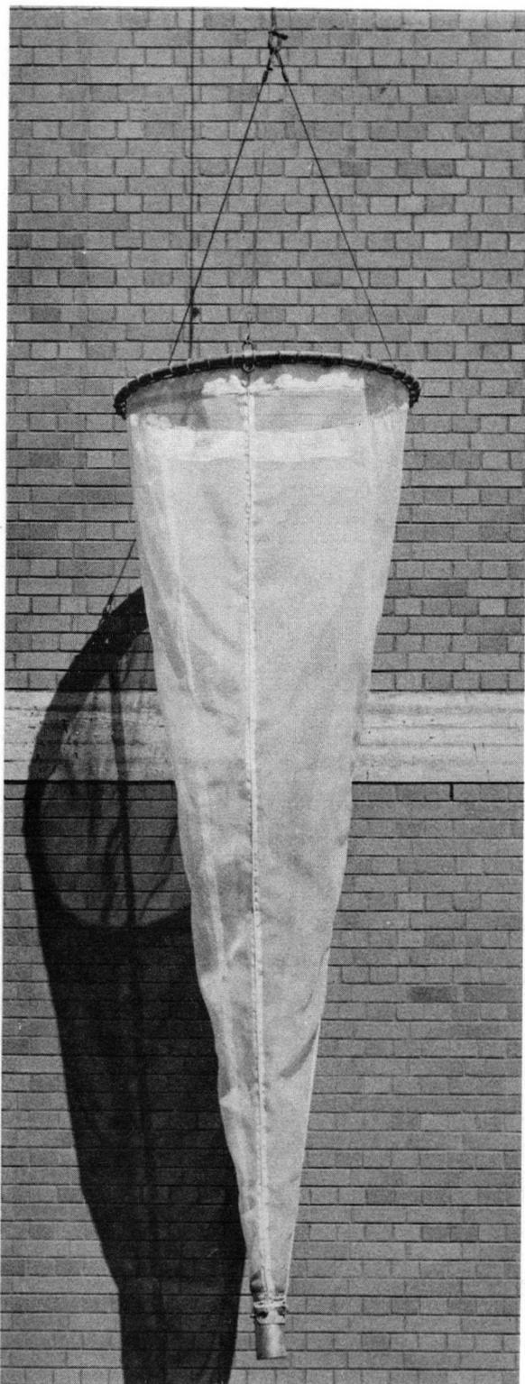
Figure 5a. The 1-metre conical sampler rigged as it was used during the field trials of August, 1965.
