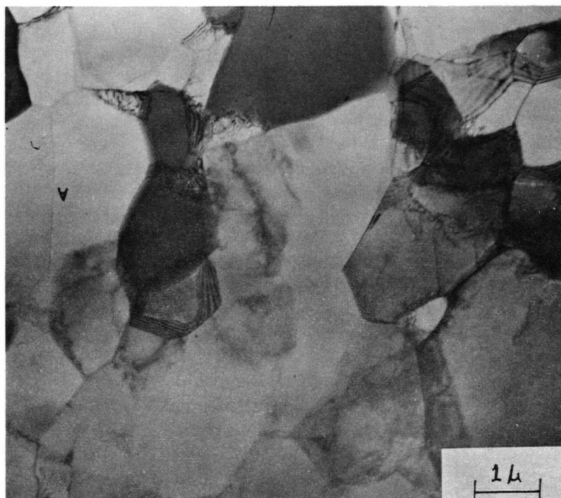
Figure 8. Transmission electron micrograph of 200°C extruded and annealed aluminum from shot.
