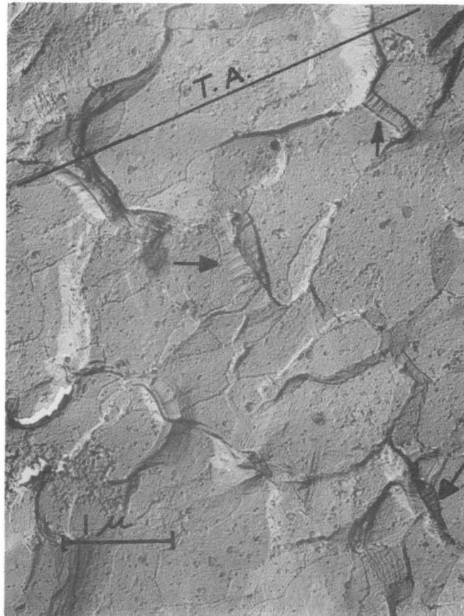
Fig. 20. As strained surface showing striated bands (marked by arrows) in grain boundary regions at 43% strain. T = +23^{\circ}\text{C} , \dot{\epsilon} = 7.8 \times 10^{-3} \text{ min.}^{-1} L_0 = 1.6 \text{ microns} .
