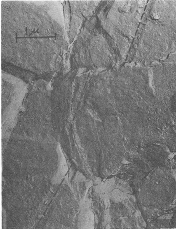
Fig. 19. Grain boundary shear and grain rotation at 43% strain. T = +23^{\circ}\text{C} , \dot{\epsilon} = 7.8 \times 10^{-3} \text{ min.}^{-1} , L_0 = 1.6 \text{ microns} .
