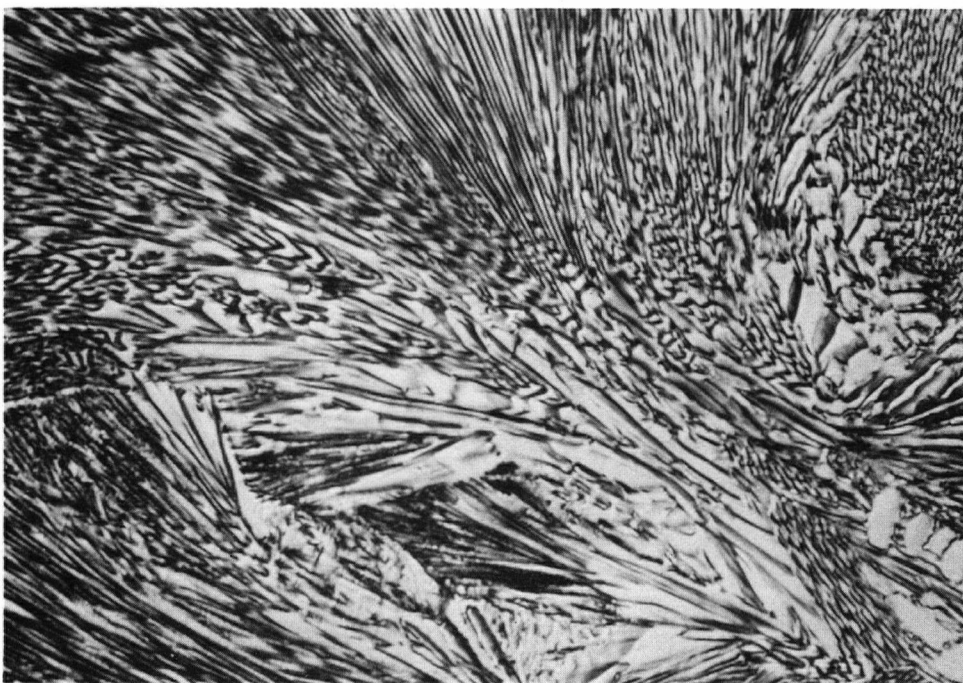
Fig. 11 Zn - 0.36 wt.% Ti alloy chill cast microstructure.
