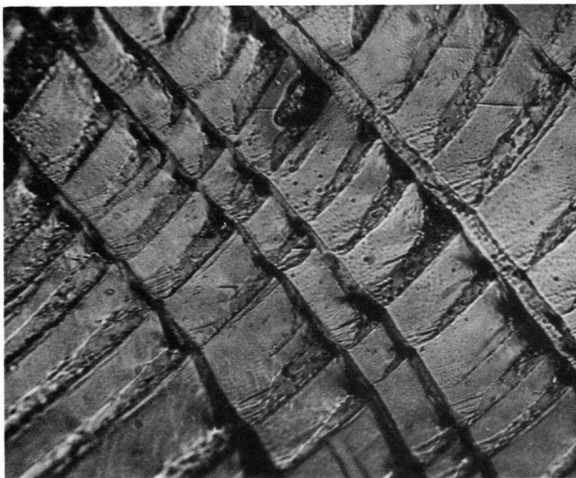
Fig 21. Intersecting twins in Nb 4.8 Ta alloy (x600).
