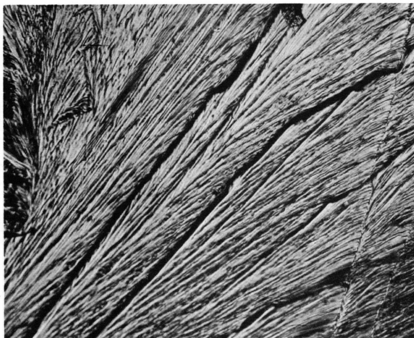
Fig 22. (001) Cleavage plane in Nb 6.6 Mo alloy (x230).
