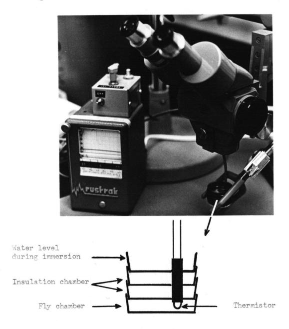
The quickest temperature changes were produced by moving the chamber from one bath to another. More gradual temperature increases were achieved by immersing the chamber in a Haake F.S. constant temperature bath and raising the bath temperature electrically.
