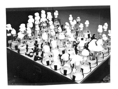
Figure 2. The horizontal shaker used for aeration of the suspension cultures - containing cultures of different ages.
