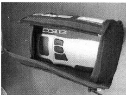
Figure A.6 SKC Leland legacy air sampling pump and noise-reducing case
