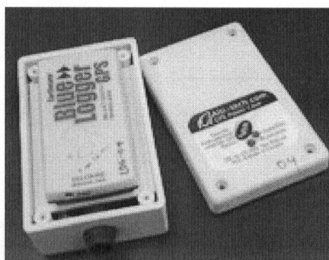
Figure A.7 GPS datalogger inside battery case
