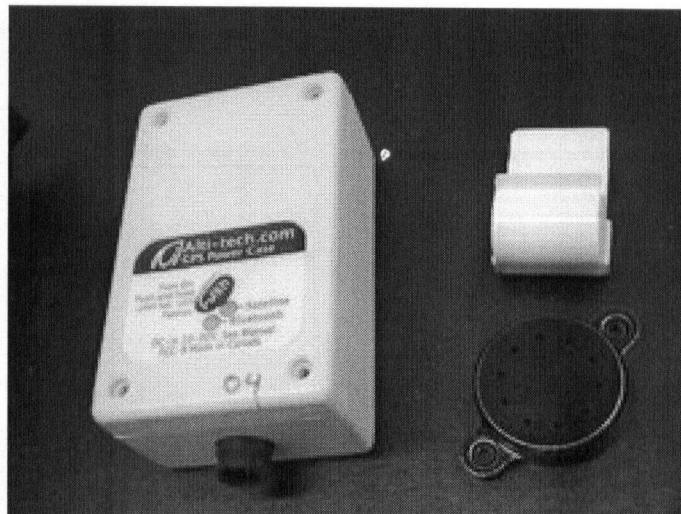
Figure A.5 GPS Datalogger case, Ogawa sampler and PEM PM 2.5 sampler head
