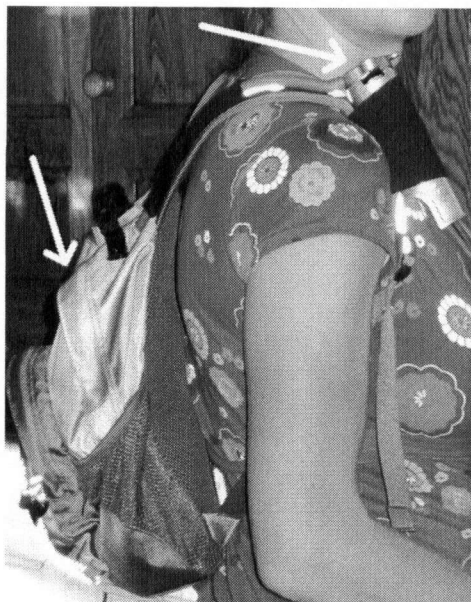
Figure A.6 SKC Leland legacy air sampling pump and noise-reducing case
